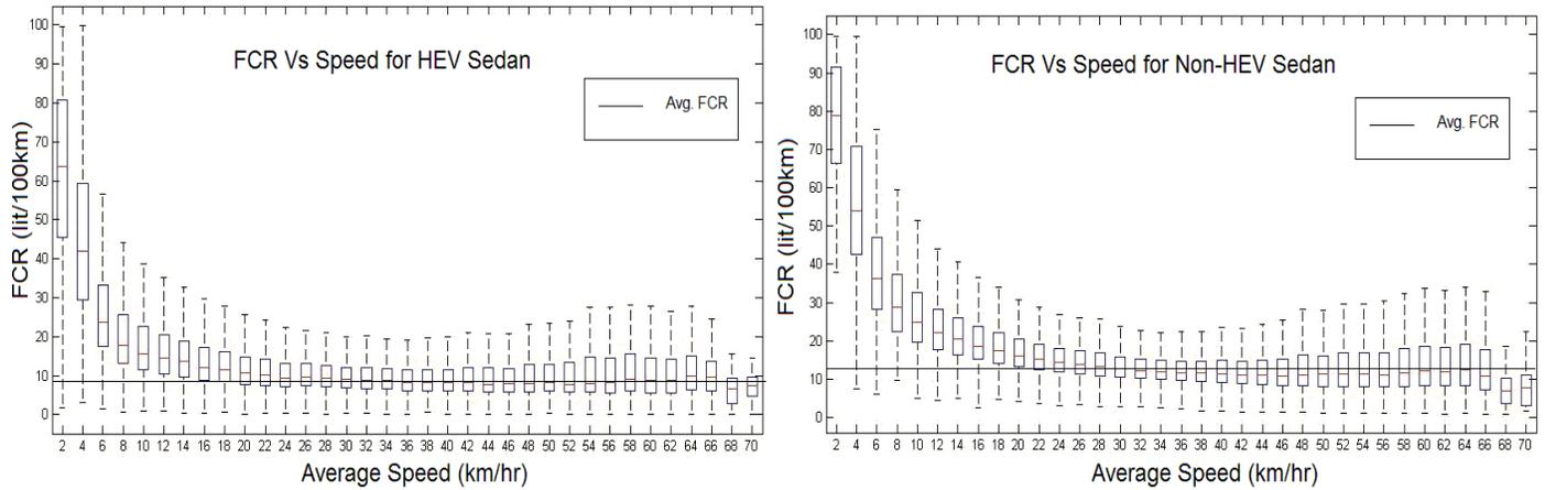
**Fig. 2:** Fuel consumption vs. speed box plot for non-HEVs and HEV sedans
