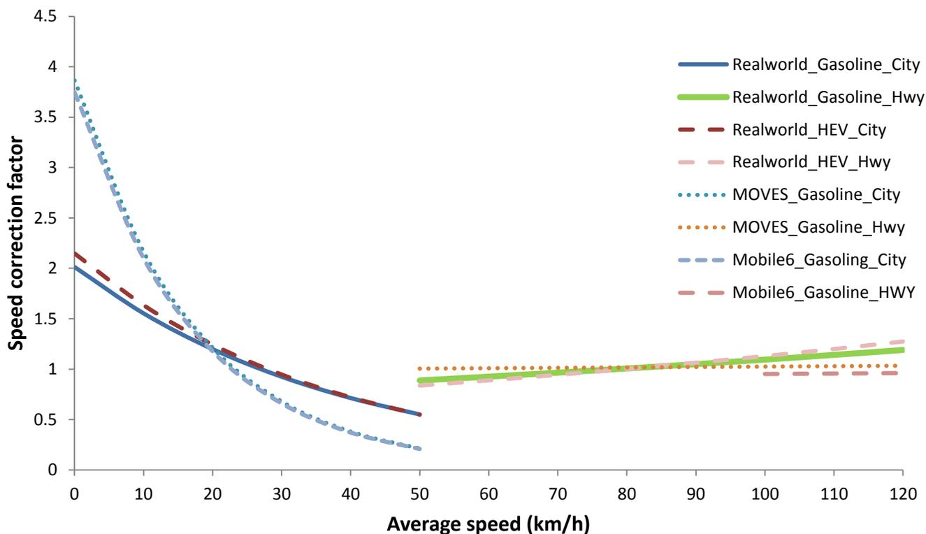
**Fig. 5:** Effect of road type and estimation methods on speed correction factor
