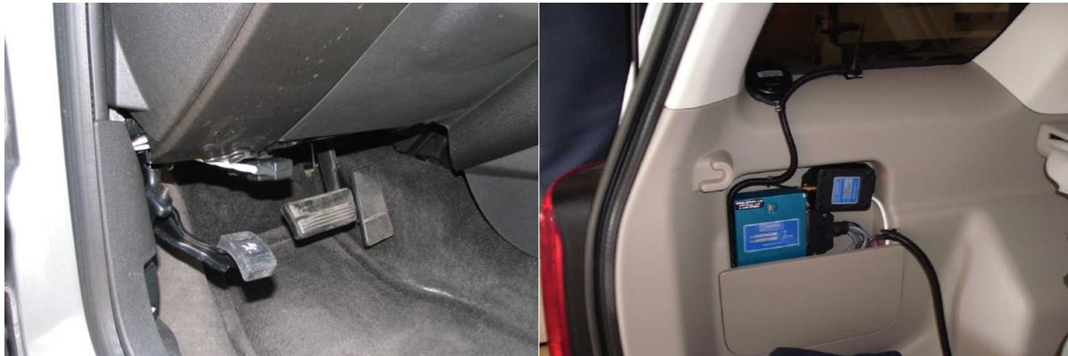
**Fig. 1:** An example of the visible data logger installed on the fleets, ISAAC instruments<sup>4</sup>
