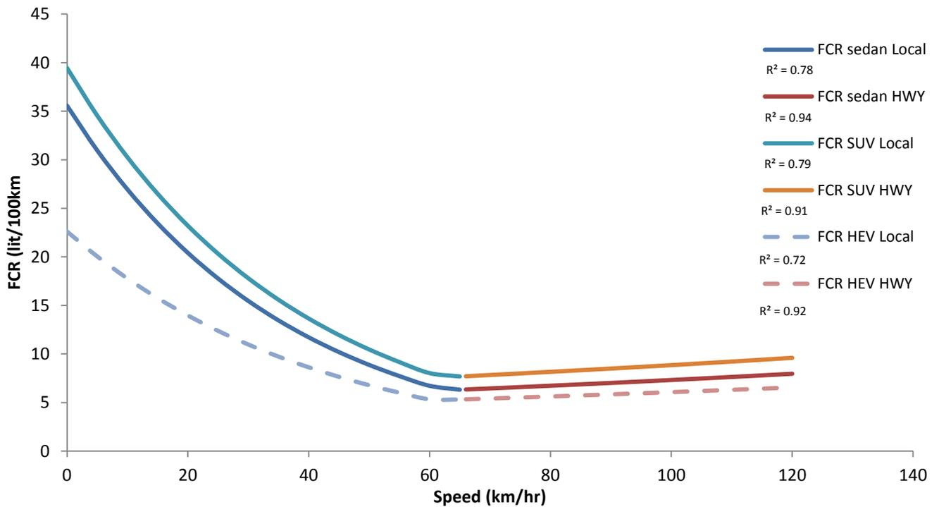
**Fig. 3:** Effect of speed and road type on FCR for different vehicle types (eco-driving study)
