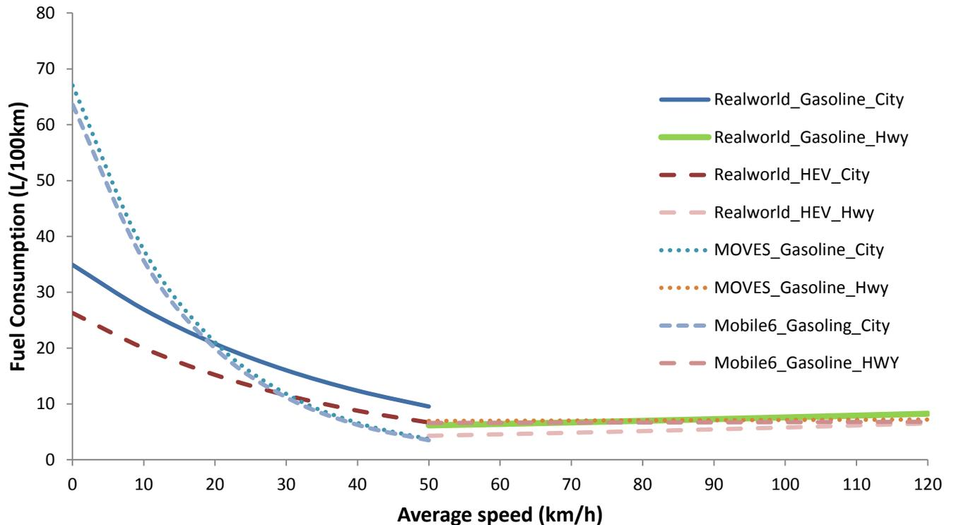
**Fig. 4:** Effect of road type and estimation methods on FCR
