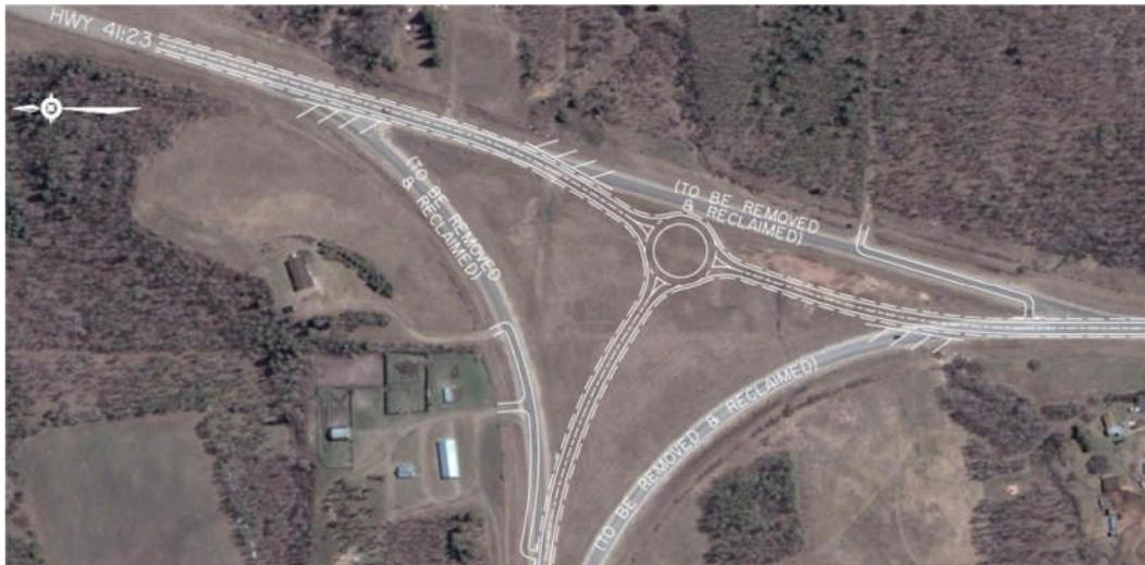
Figure 9 Conceptual design of single-lane roundabout
