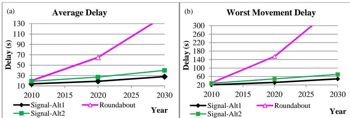
Figure 7 Average delays and delays on the worst movement
