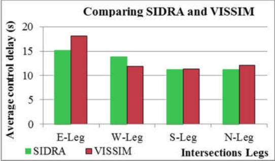
Figure 4 Approach delay comparison between SIDRA and VISSIM
