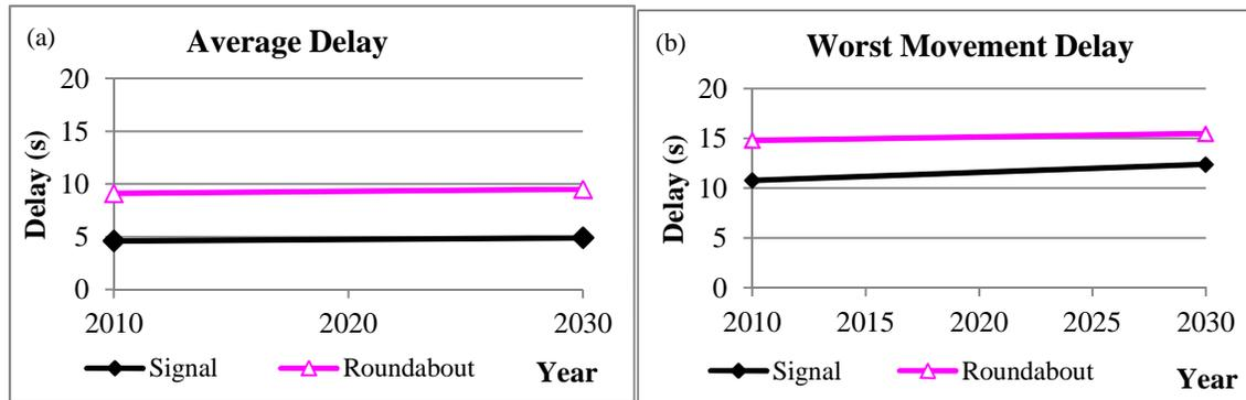
Figure 10 Average delay and delay of the worst movement
