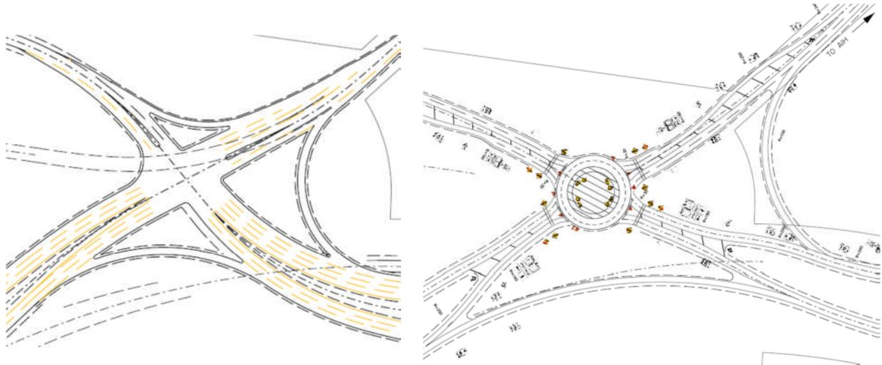
Figure 6 Conceptual designs for channelized intersection and roundabout
