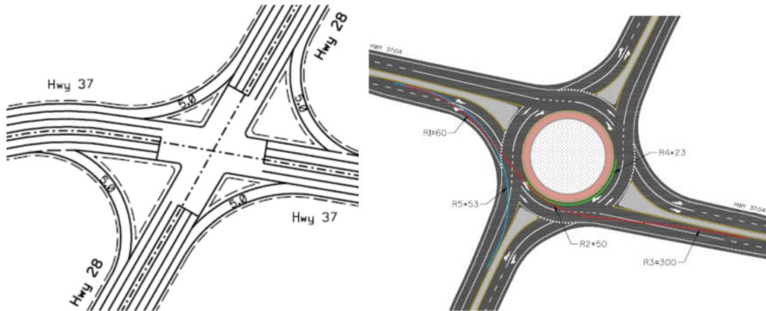
Figure 2 Channelized intersection and roundabout
