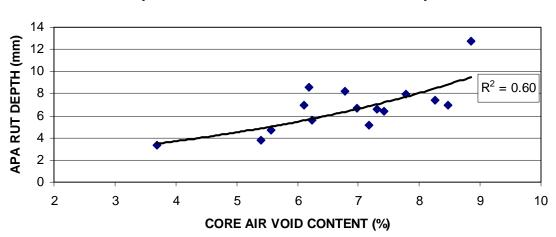
Figure 4 Comparison of Core Air Voids and Rut Depth
