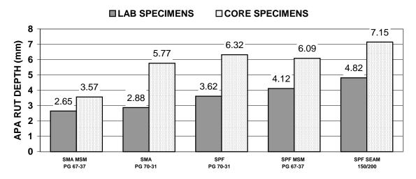
The lab prepared samples appear to not only have less variability than field core specimens, but appear to better discriminate between mixture types. A comparison of these results indicates a clear superiority of SMA mixtures in terms of rutting performance. This is consistent with previous evaluations of rut resistant HMA materials.
