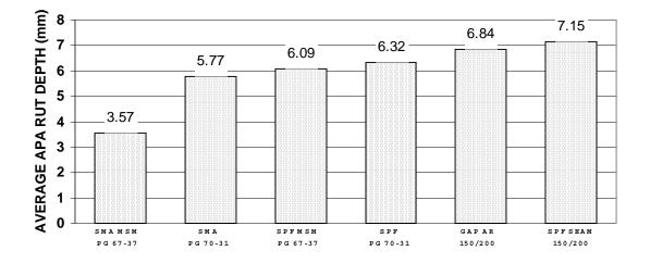
Figure 3 APA Ranking Based on Field Core Testing
