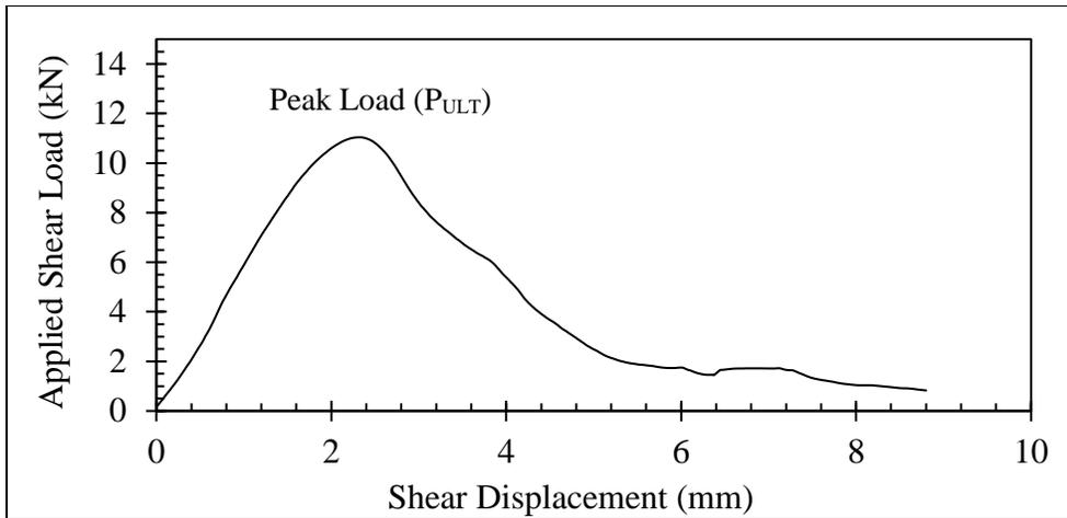
**Figure 2-8 Typical Shear Load-Displacement Curve**
