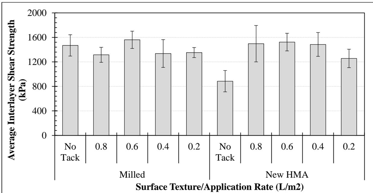
**Figure 3-1 Interlayer Shear Strength (ISS) Results**
