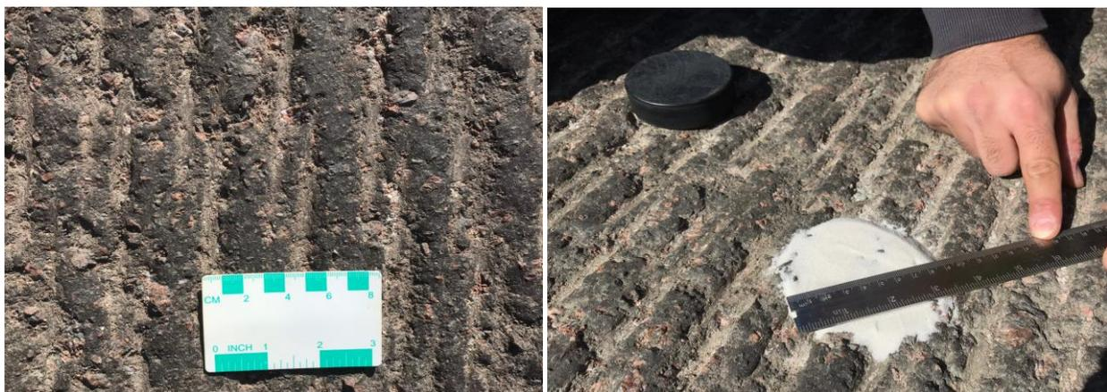
**Figure 2-2 Milled Texture Prior to Application of Tack Coat (Left) and Measurement of Texture Depth Using the Sand Patch Test (Right)**
