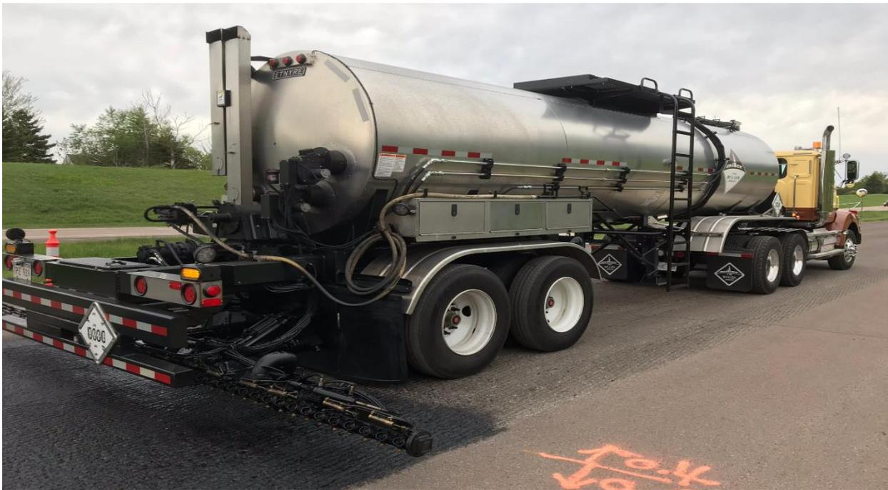
**Figure 2-3 Etnyre Distributor Truck Used for the Study**
