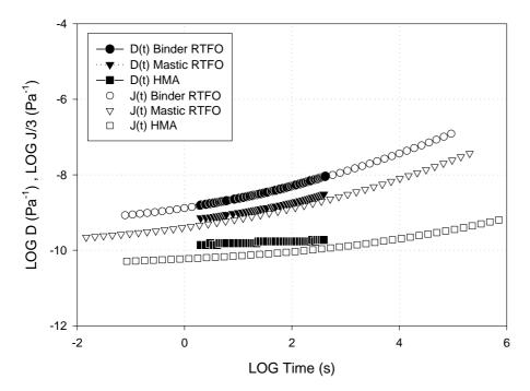
**Figure 6.** Comparison of the shear (J/3) and creep (D) moduli at -28  $^{\circ}C$
