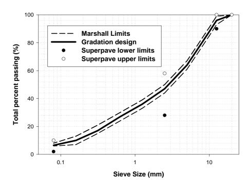
Figure 1. Hot mix asphalt grain size distribution curve
