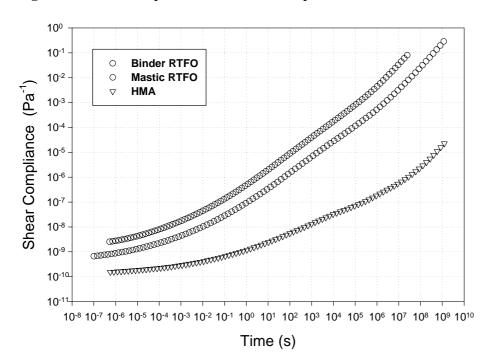
**Figure 5.** Shear compliance calculated via spectra at  $T_{ref.} 0$  °C
