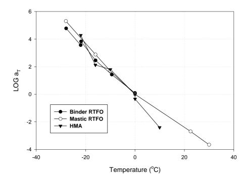
Figure 3. Horizontal shift factor a<sub>T</sub> of asphalt binder, mastic and hot mix asphalt
