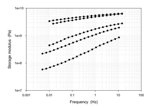
Figure 2. Hot mix asphalt isochrones of storage modulus (G') at temperature range  $10 \sim -22$  °C
