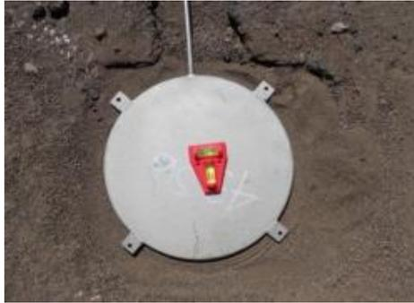
**Figure 4. Earth Pressure Cell [32]**
