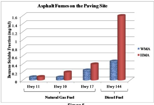
Figure 5 -Asphalt emissions on the paving site behind the paver
