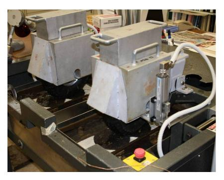
Figure 6 - MTO's modified Hamburg wheel track testing machine equipped with pneumatic tires
