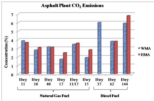
Figure 2 -Carbon dioxide emissions at the asphalt plants
