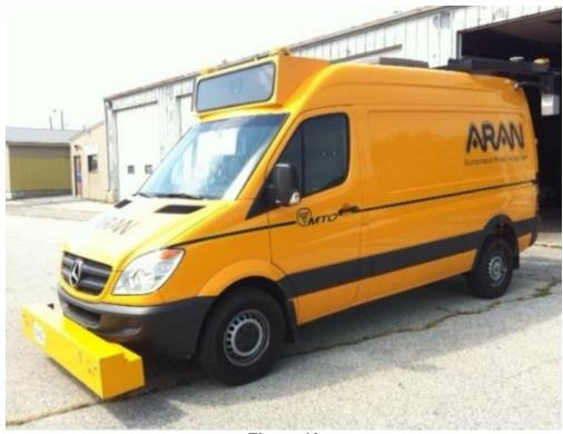
Figure 10 – Latest generation of MTO's ARAN (Automated Road ANalyzer)
