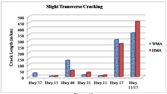
Figure 13 – Extent of slight severity transverse cracking on the WMA and HMA sections
