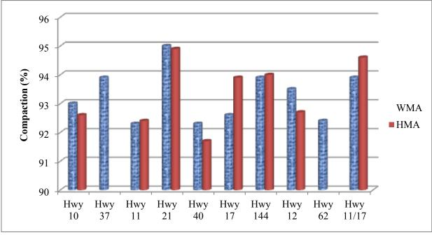
Figure 8 – Average field compaction results
