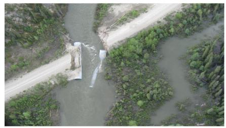
Figure 3: Aerial View of Highway#10 after washout Km74
