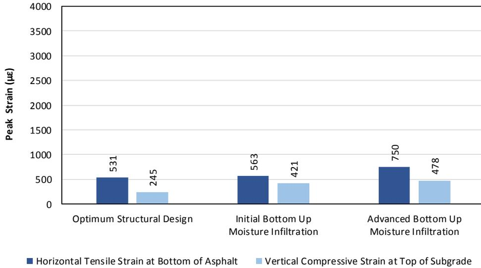
**Figure 7 Peak Conventional Orthogonal Strains by Moisture Condition**
