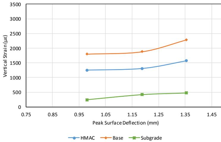
**Figure 13** Peak Vertical Compressive Strain versus Peak Surface Deflection
