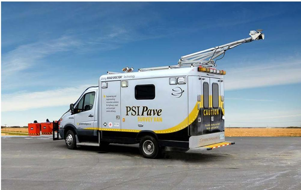
**Figure 3** Surveying van with GPR, Lidar and Video Camera
