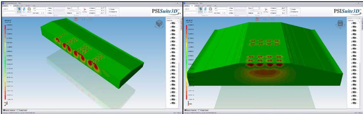
b) Loading with Two B-Trains – Initial Bottom Up Moisture Infiltration in Prepared Subgrade
