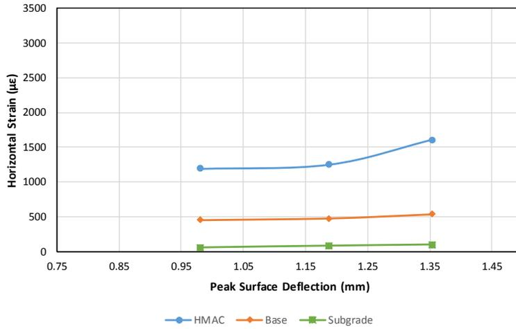
**Figure 12** Peak Horizontal Tensile Strain versus Peak Surface Deflection
