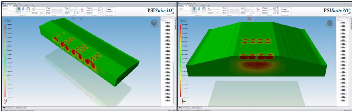
c) Loading with Two B-Trains – Advanced Bottom Up Moisture Infiltration into Structural Layers
