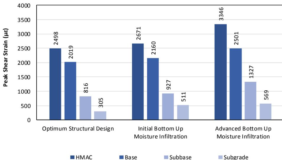
**Figure 8 Peak Shear Strain – by Layer by Moisture Condition**
