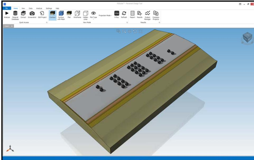
Figure 2 Example of Numerical Model Mesh Illustrating Two B-Trains Passing
