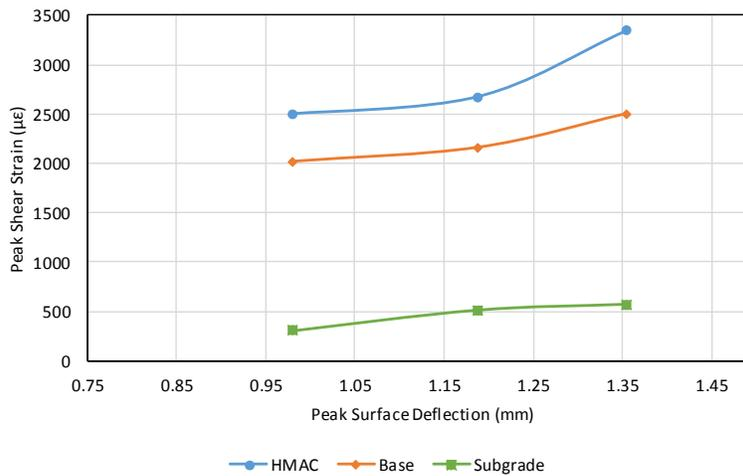
**Figure 14** Peak Shear Strain versus Peak Surface Deflection
