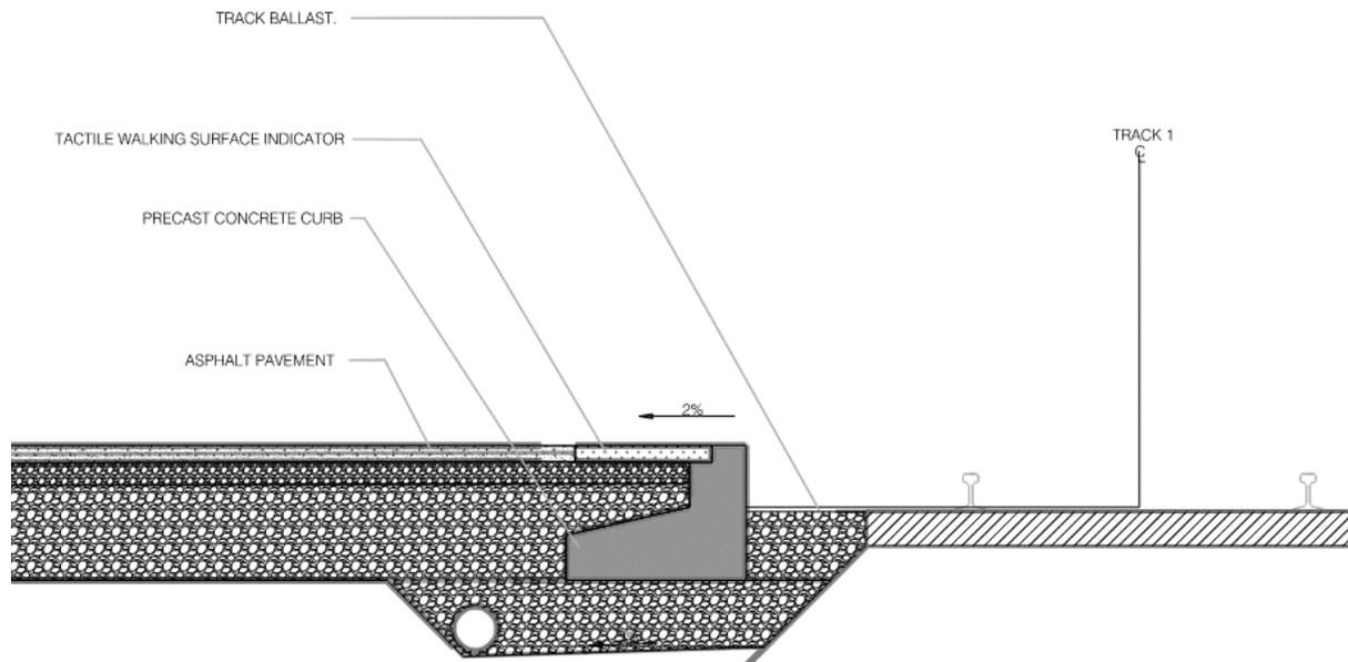
Figure 5 - Section cut of the new platform
