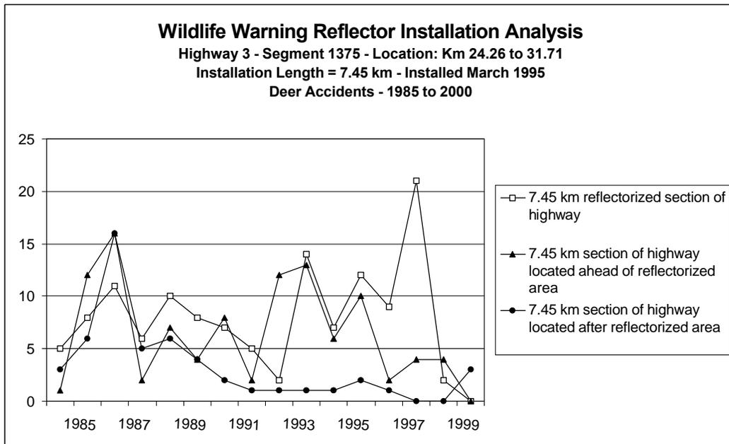
Figure 7. Wildlife warning reflector installation analysis (Highway 3, Segment 1375)
