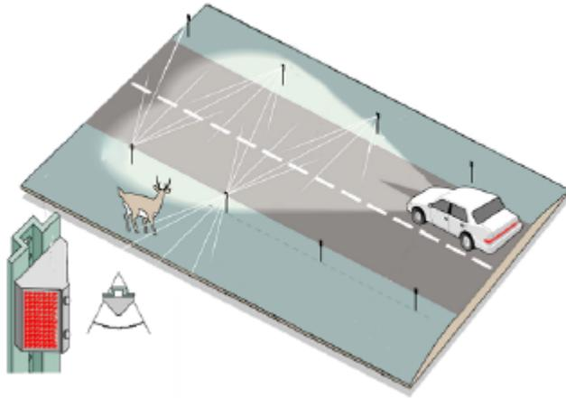
Figure 4. Light reflection concept of wildlife warning reflectors
