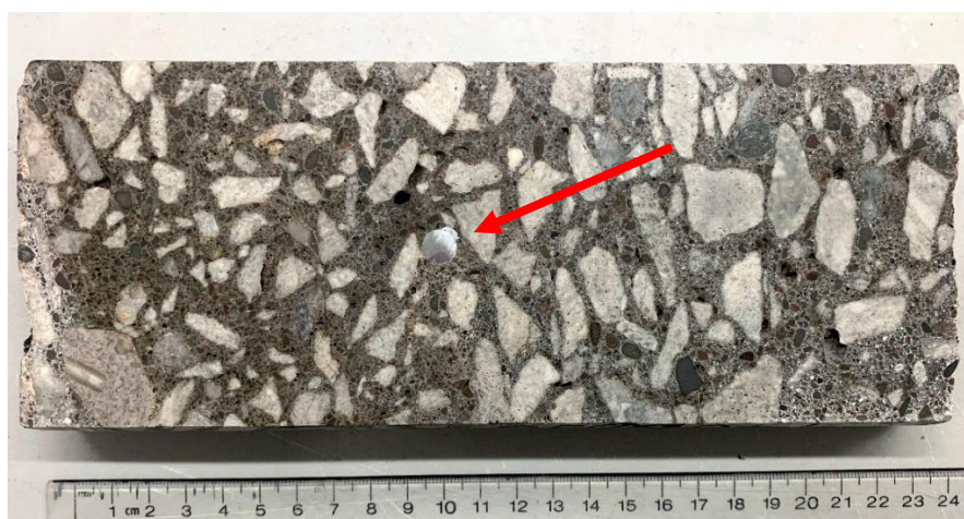
Figure 11: Prepared concrete core with clean uncorroded mesh
