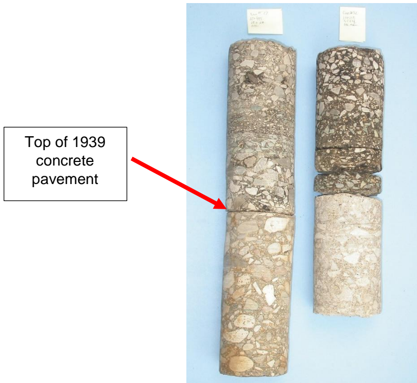
Figure 10: Cores through composite pavement showing very good quality 65-year-old concrete.
