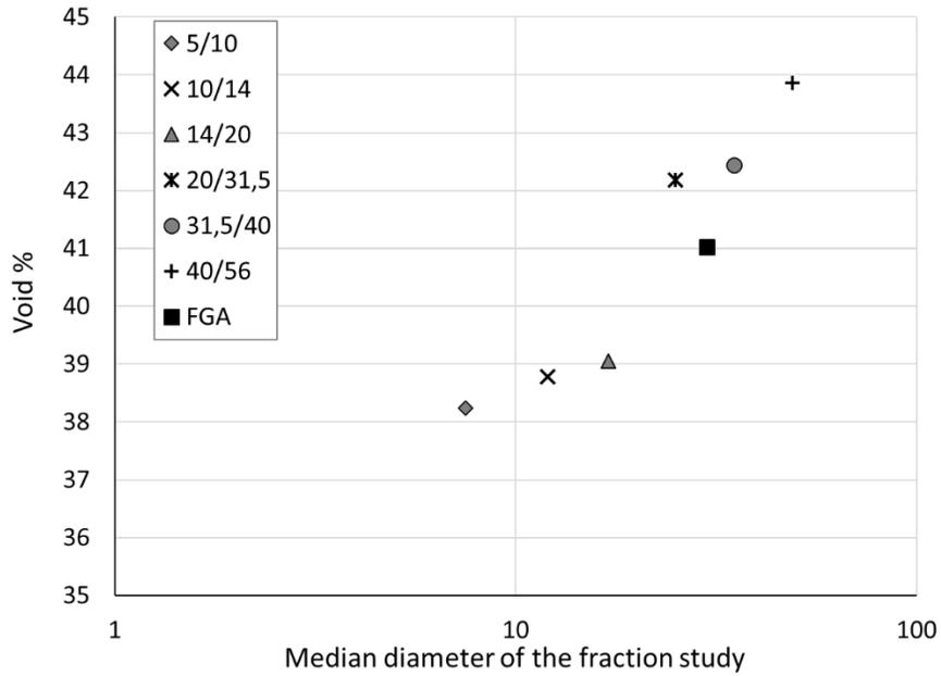
Figure 3 : Void percentage with respect to particle size range of compacted FGAs (minimal diameter / maximal diameter) [LC 21-060].
