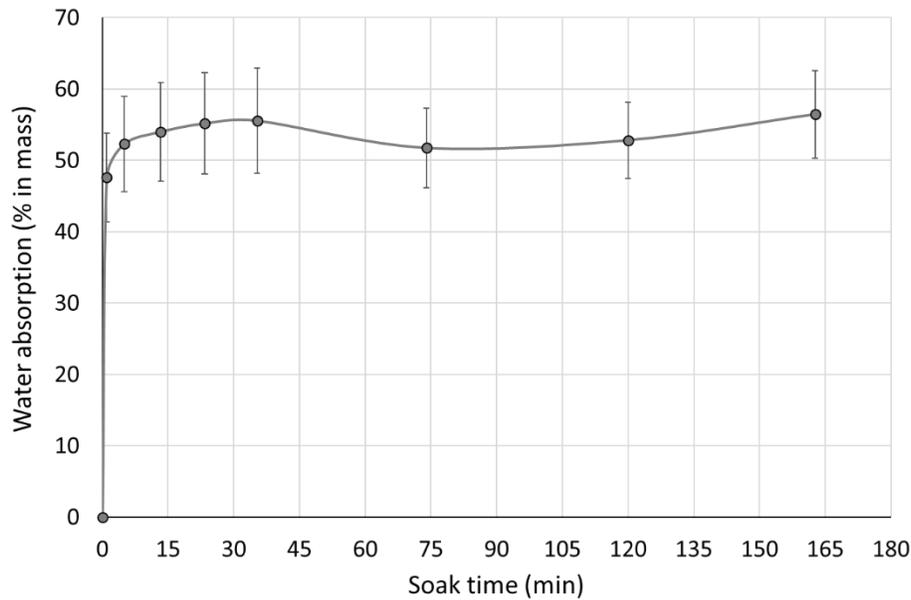
Figure 4 : FGA's water absorption as a function of time.
