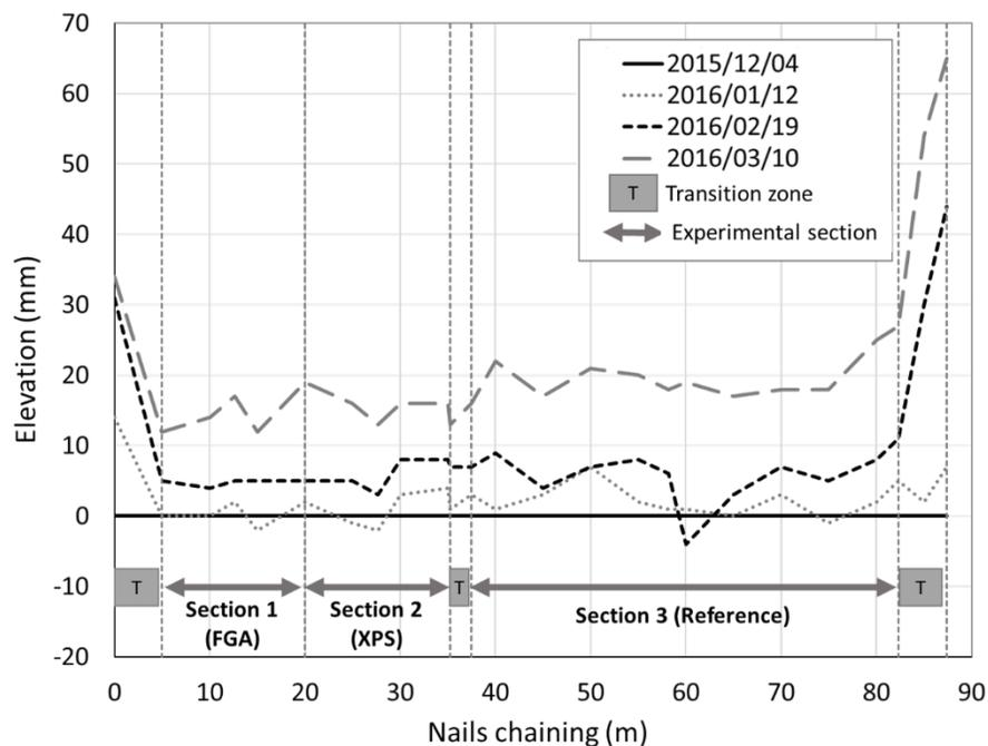
Figure 7 : Elevation (mm) of the road at the Kingsey Falls test site
