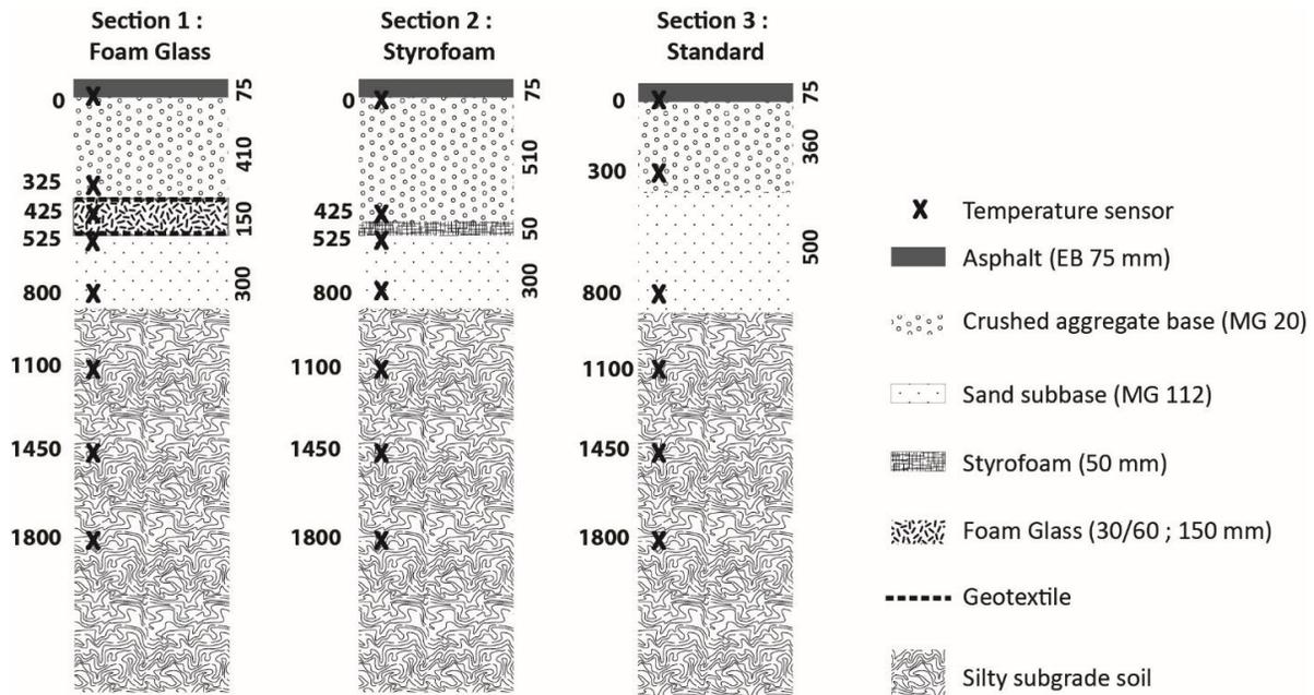
Figure 5 : Description of each test section (layer composition and thickness and temperature sensor position - dimensions in mm).
