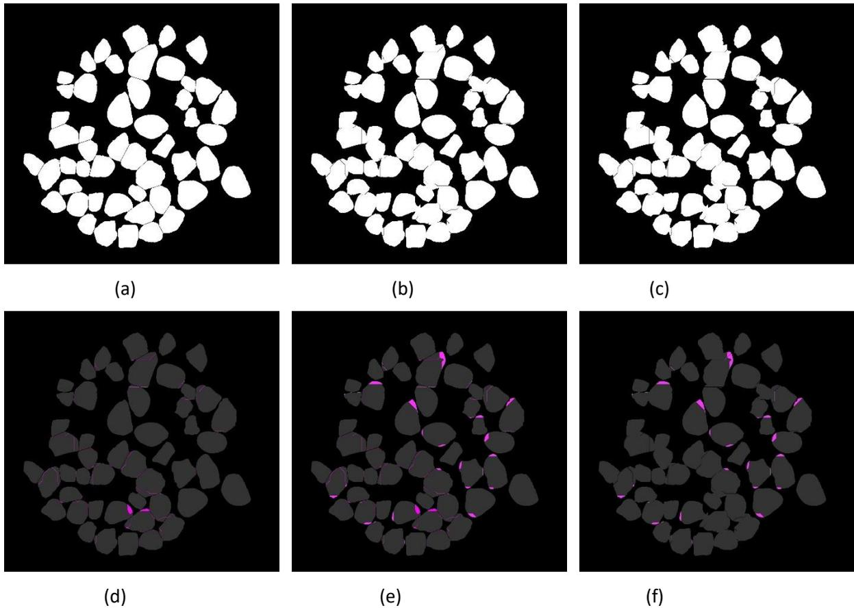
**Figure 7 Effect of segmentation methods: (a) Manual segmentation based on corner points, (b) Partial segmentation based on EMT, (c) Global segmentation based on EMT, (d) composite of Manual**
