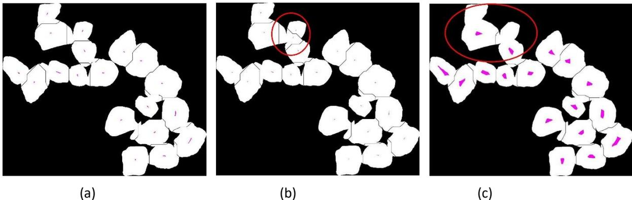
**Figure 6 Segregation Results: (a) correct-segmentation, (b) over-segmentation, (c) insufficient-segmentation**
