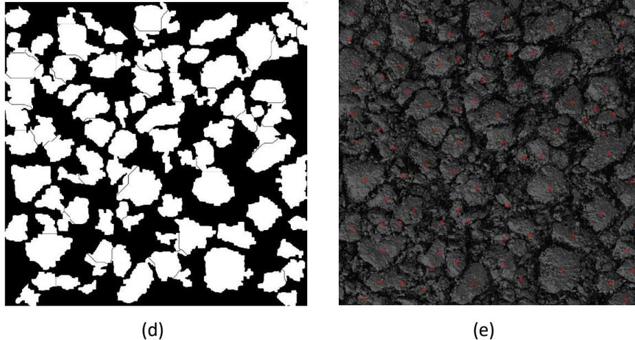
**Figure 9. Watershed Segmentation Results of Loose Asphalt Mixture based on EMT: (a) Original asphalt mixture, (b) Composite image with whole identified particles, (c) Composite image with identified particles larger than 4.75mm, (d) Segmentation result of identified particles larger than 4.74mm, (e) Marked grayscale image**
