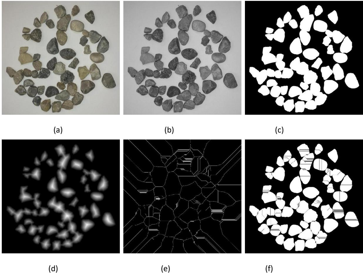
**Figure 1 Watershed segmentation transform steps: (a) original RGB image, (b) grayscale image, (c) binary image, (d) distance-transformed image, (e) watershed ridgeline, (f) final result of watershed segmentation.**
