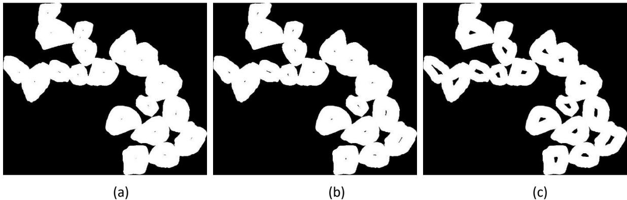
**Figure 4 Regional maxima result with different threshold  $h$ : (a)  $h = 0.01$ , (b)  $h = 0.02$ , (c)  $h = 0.05$**
