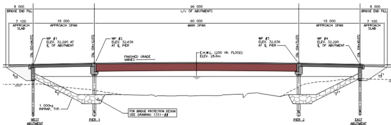
Figure 1: Original design concept: Composite steel plate girders in the main span and precast pretensioned concrete box girders for the approach spans [BC MoTI]
