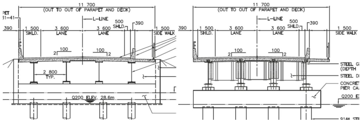
Figure 3: Final design concept: Cross Sections at the abutment (left) and at the pier (right) [BC MoTI]
