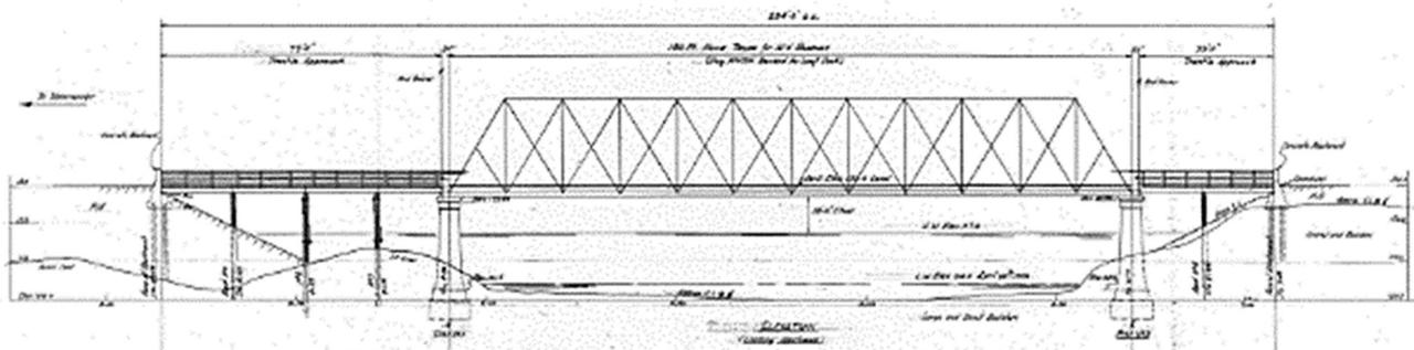
Figure 12: Old Chehalis Bridge: Timber Howe Truss with timber approach spans [BC MoTI]
