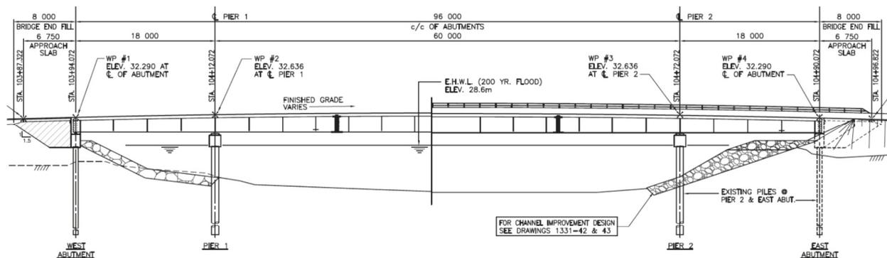
Figure 2: Final design concept: Continuous composite steel plate girders over the entire length of the bridge [BC MoTI]
