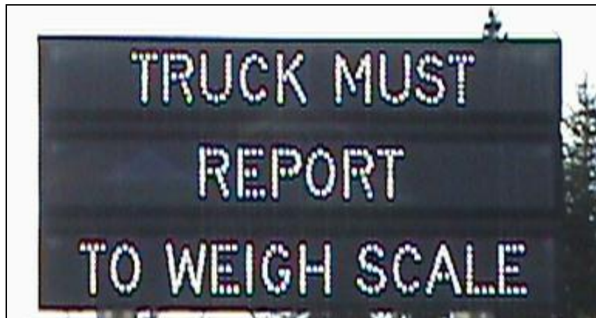
Figure 13 Implementation of a Changeable Message Sign
