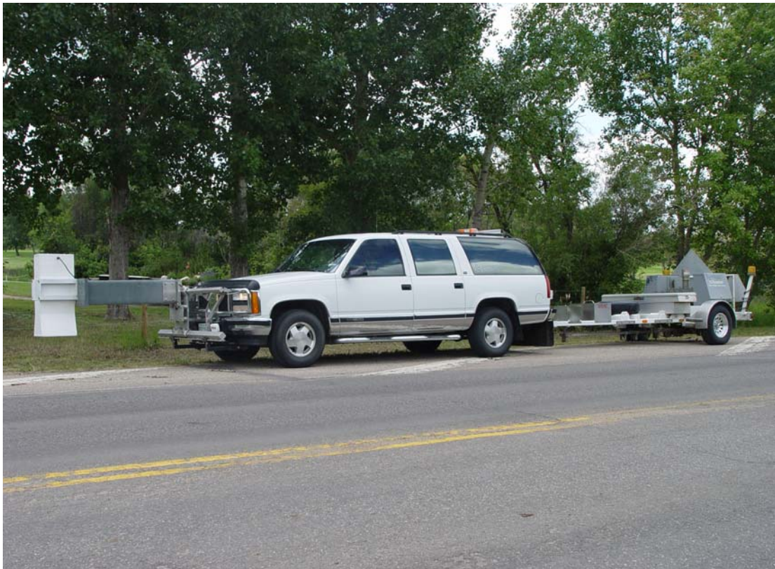
Figure 4.1 PSI Technologies Ground Penetrating Radar and Falling Weight Deflectometer
