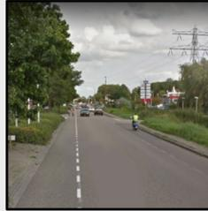
**Advisory Bike Lanes:** Advisory bike lanes run on both sides of a single, bi-directional, vehicle travel lane. They are marked by a dashed line which permits opposing motor vehicles to enter the advisory bike lane temporarily when safe to do so to pass a vehicle moving in the opposite direction.
