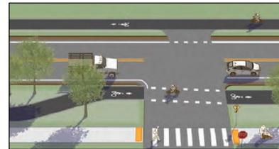
Bend-out intersection approaches shift the bicycle lane away from the intersection to create space for turning vehicles to wait for bicyclists without impeding other vehicle traffic.
