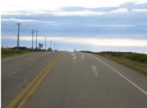
Vertical crest curves can impose significant sight constraints. Along routes through rolling terrain, there may be several locations where stops are located in the vicinity of crest curves, with insufficient sight distance. Sag curves may also create sight obstructions during dark conditions.
