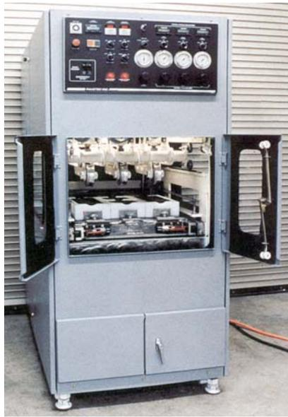
**Figure I Asphalt Pavement Analyzer**
