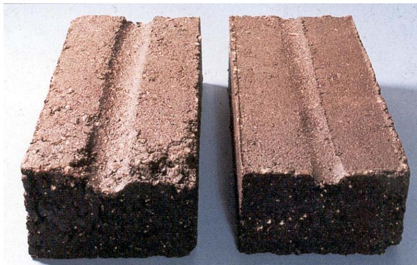
**Figure VII Tested Beam Samples in APA**
