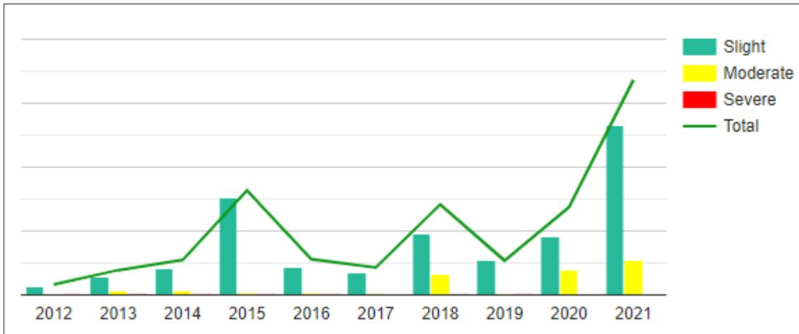
Figure 10. 2012 to 2021 Total Crack Area (Alligator) for Combined CIR and CIREAM Sections
