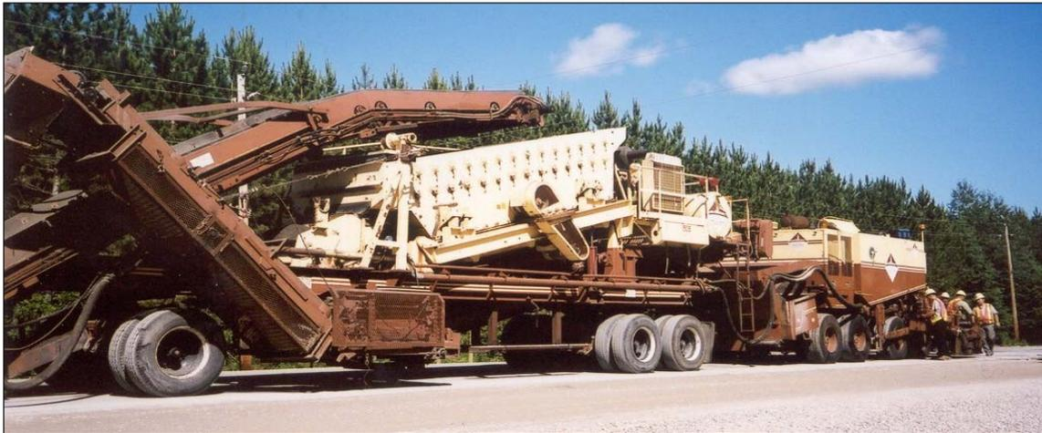
Figure 2. Cold-In-Place Recycling Train
