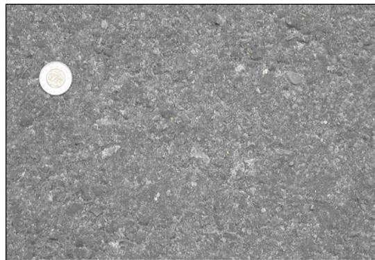
**Figure 4. a) Finished Surface of CIR Mix**
