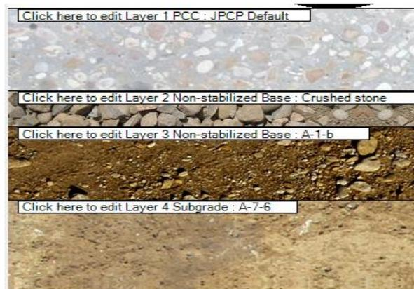
Figure 2: Typical Manitoba JPCP pavement structure (instance of Class C1)
