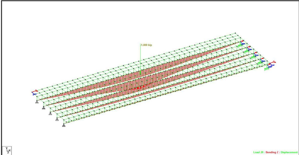
**Fig. 9 – Virtis 3D Model of the I-Girder Bridge. Note the Bending Moment Envelope for a Unit Load Placed on a Beam Node.**
