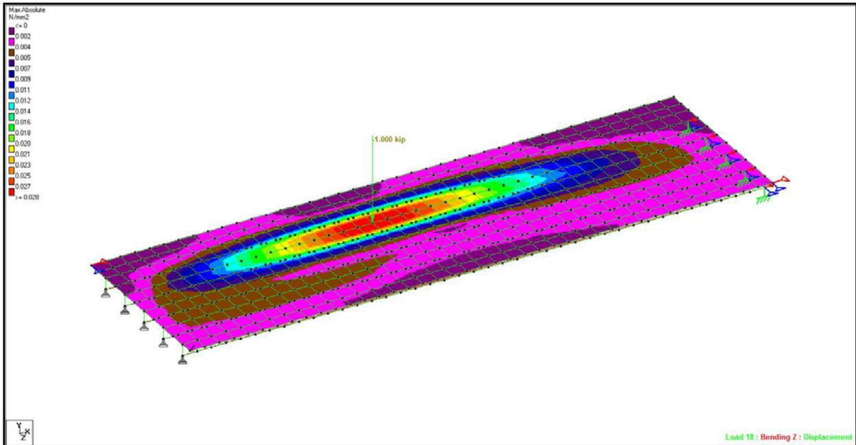
**Fig. 10 – I-Girder Bridge 3D Stress Influence Surface for the unit Load Case No. 12, Placed at a Shell Node.**
