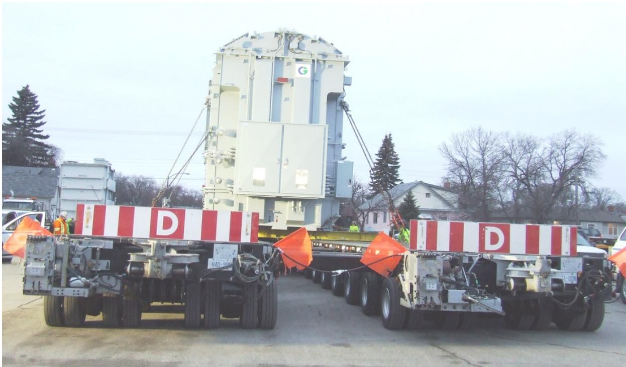
***Fig. 1 – 357 000 Kg Superload on Dual Lane 20-Line PST Hydraulic Trailer with 8 Wheels per Axle***
