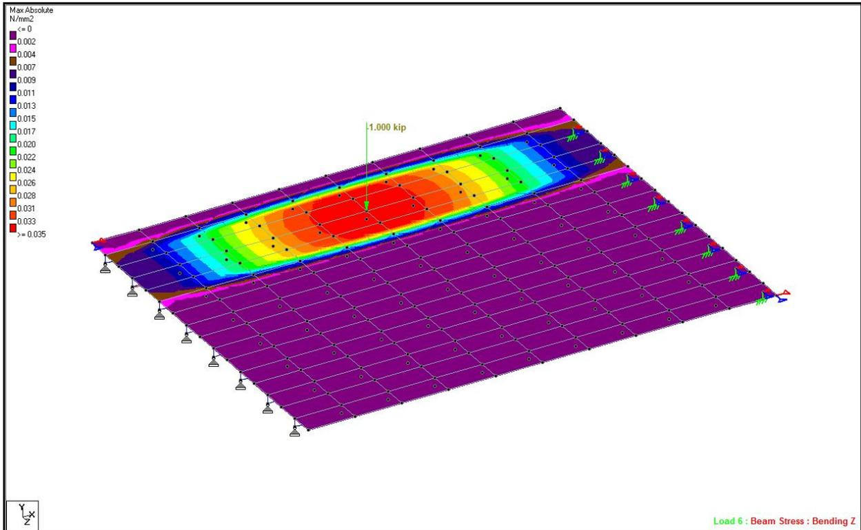
**Fig. 8 – PPCC Bridge 3D Stress Influence Surface for the unit Load Case No. 6, Placed at a Shell Node.**
