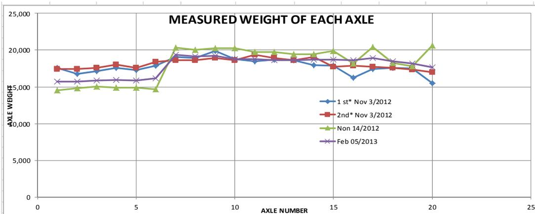
**Graph No. 3 - Measured Axle Weights Prior to Issuing Each Overload Permit.**
