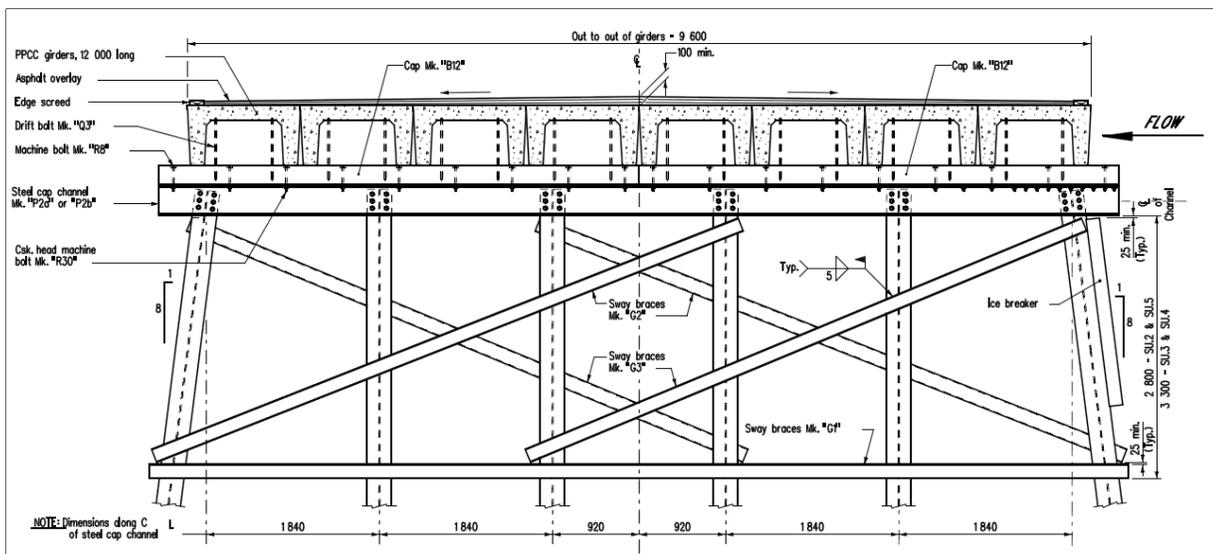
**Fig. 4 - St. Adolphe Coulee PPCC Bridge Cross-Section**
