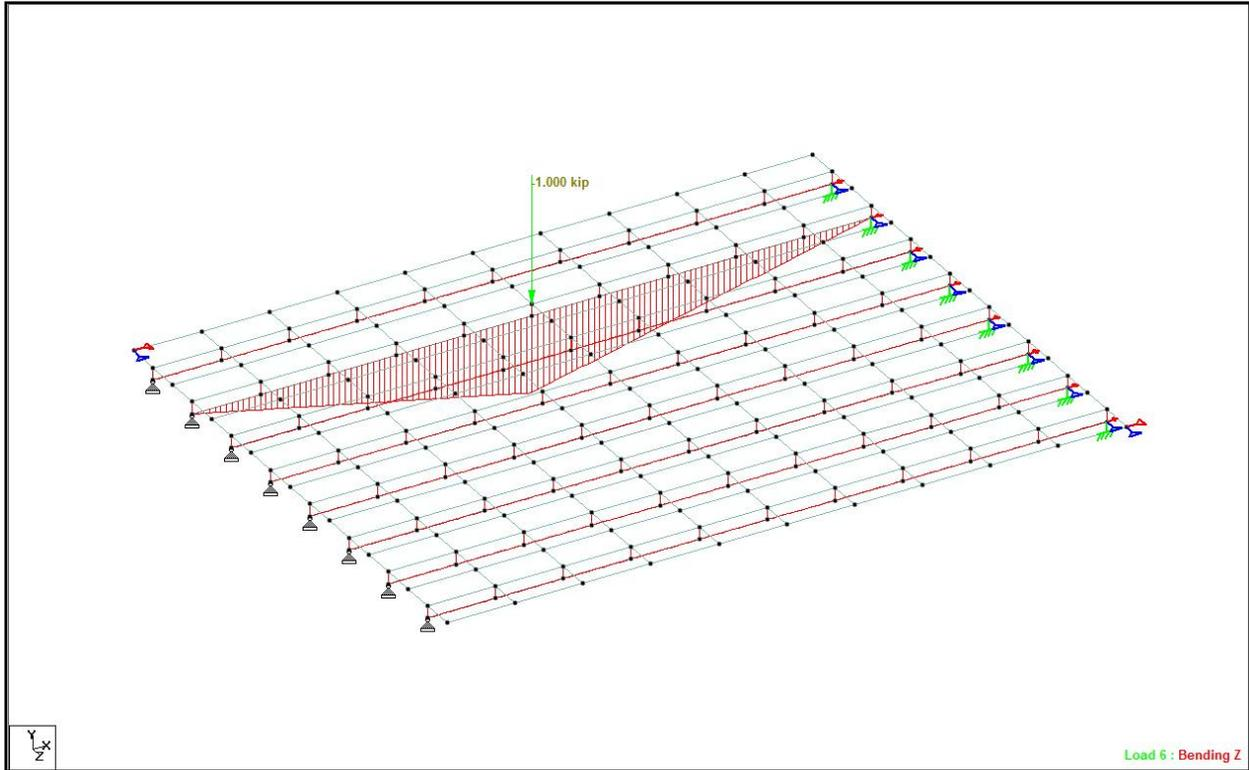
**Fig. 7 – Virtis 3D Model of the PPCC Bridge. Note the Bending Moment Envelope for a Unit Load Placed on a Beam Node.**
