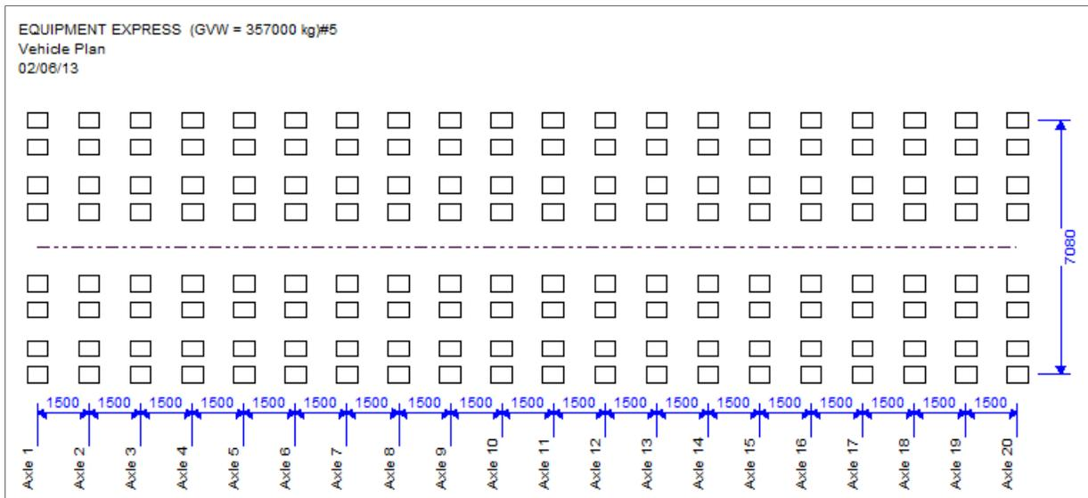
**Fig. 5- Graphical outputs for the transverse and longitudinal configuration of the proposed trailer**
