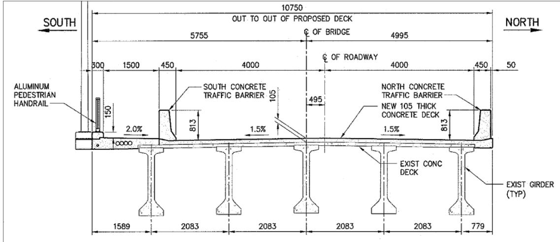
**Fig. 3 - Red River I-Girder Bridge Cross-Section**
