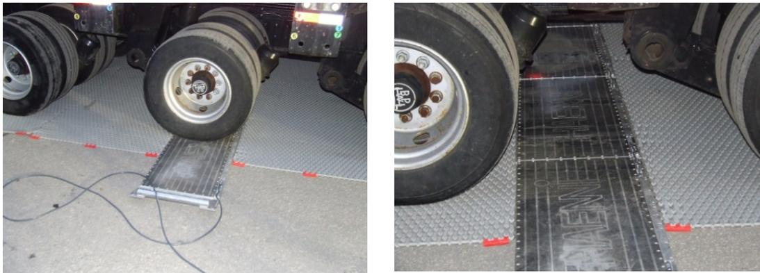
**Fig. 11 - Weighing All Trailer Axles Using Portable Scales Prior to Issuing each Permit.**
