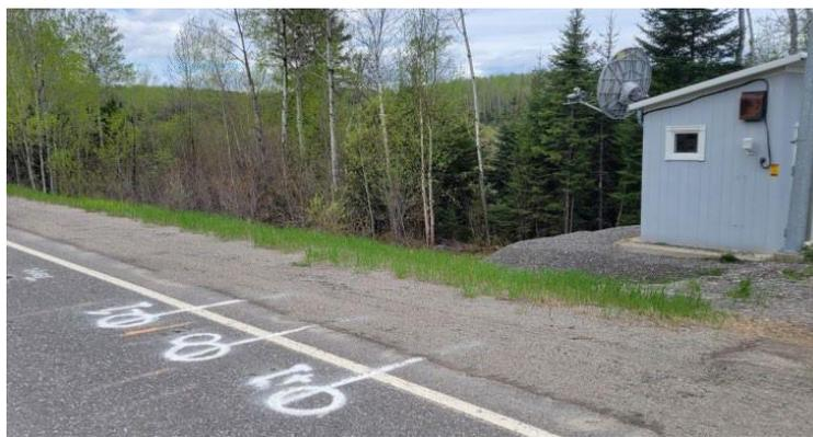
Figure 7. Example of FWD Testing Location along the Wheelpath
