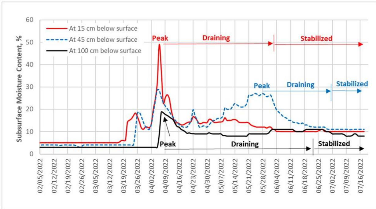
Figure 6. Example of Daily Subsurface Moisture Content Drainage Trend (Hwy 599)
