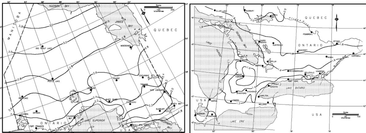
Figure 3. Foundation Frost Penetration Depths for Northern (left) and Southern (right) Ontario
