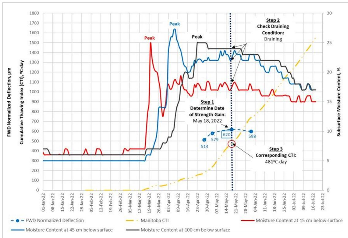
**Figure 10. Example of RLP CTI End Date Determination Results (Hwy 671)**
