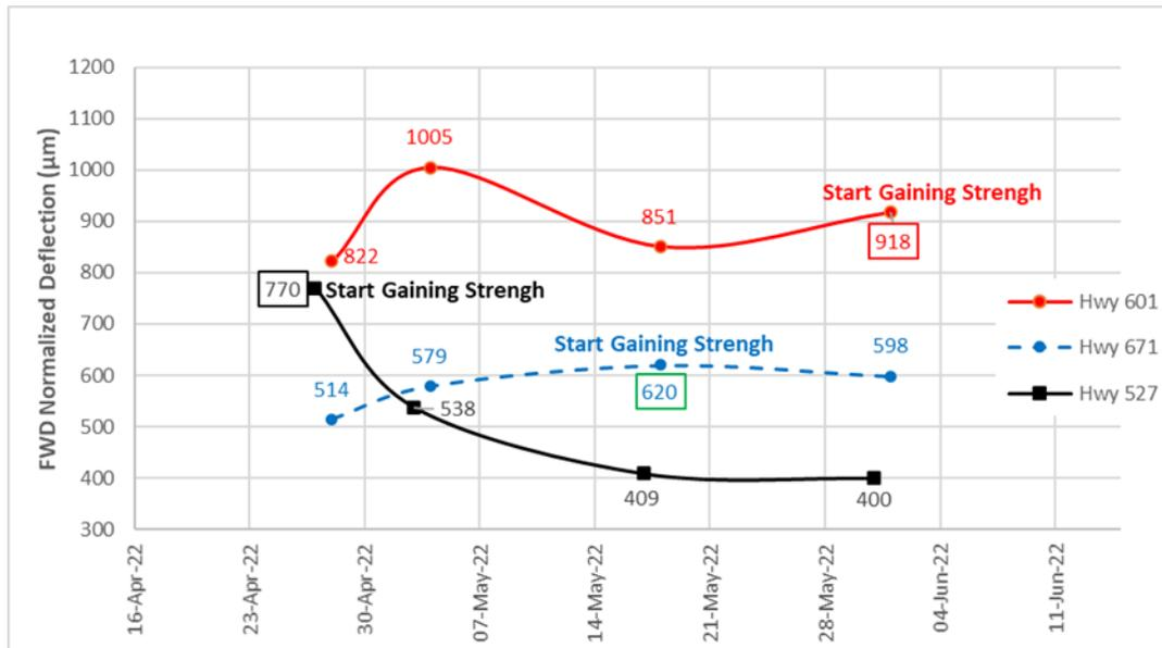
**Figure 8. Example of Pavement Strength Recovery Trends**
