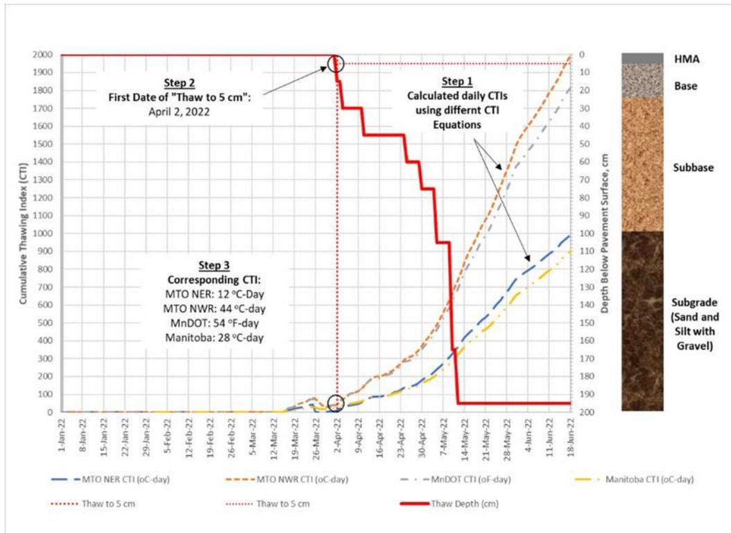
**Figure 9. Example of RLP CTI Start Date Determination Results from Steps 1 to 3 (Hwy 527)**
