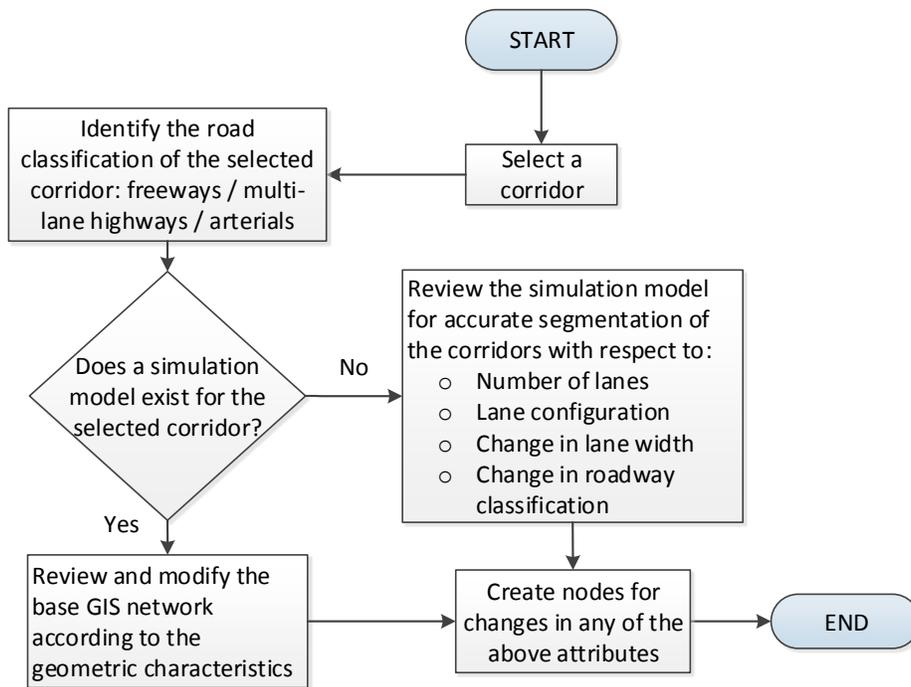
**Figure 1: Flowchart of Segmentation for Micro Level**
