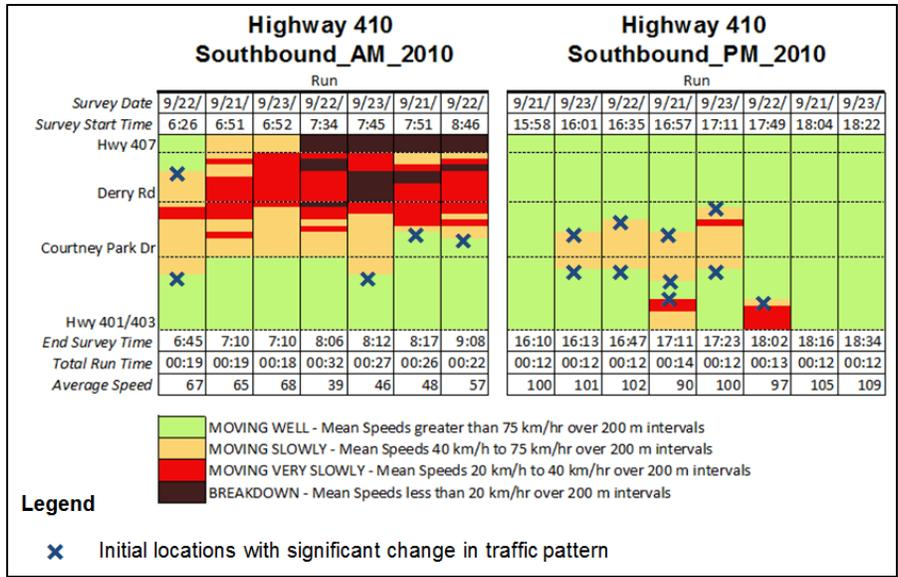
Figure 5: Initial Nodes from Speed Diagram (Highway 410 Southbound)
