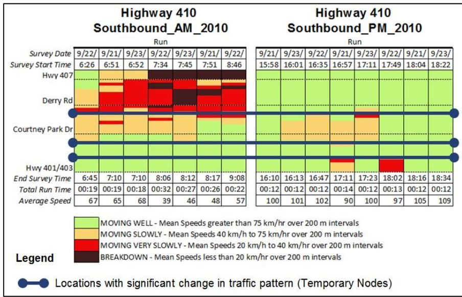
Figure 6: Temporary Nodes from Speed Diagram (Highway 410 Southbound)
