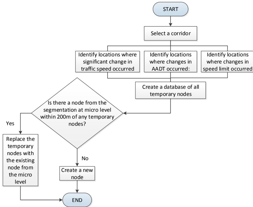
**Figure 2: Flowchart of Segmentation for Meso Level**
