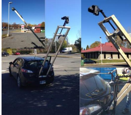
**Figure 2:** The utilized IR camera (FLIR T650sc) mounted on a vehicle.
