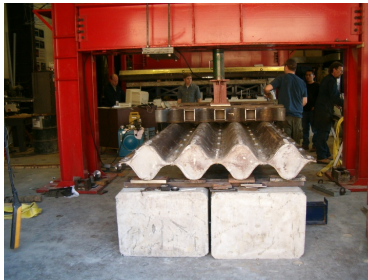
Figure 13. Flexural testing of encased concrete rib specimen
