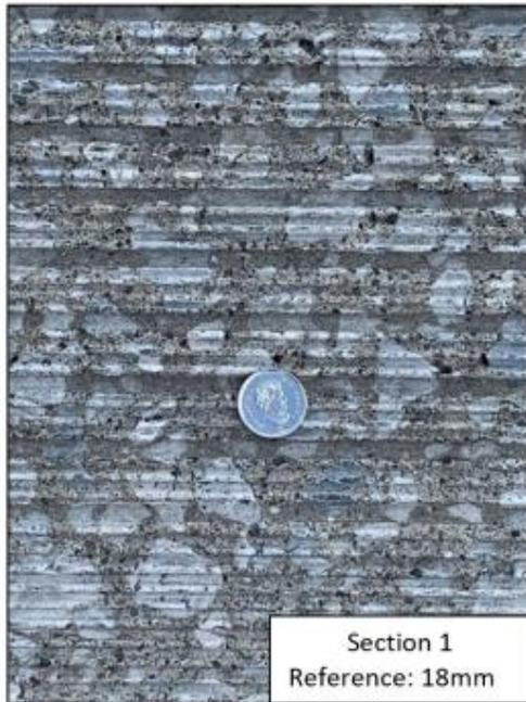
Concrete – Longitudinally grooved
