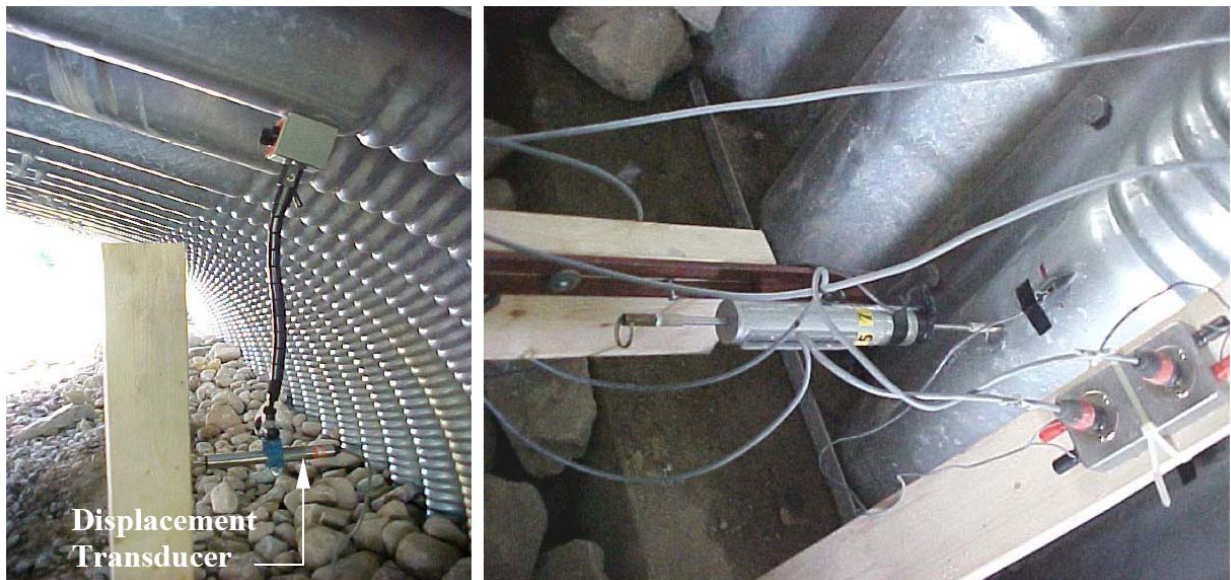
Figure 9: Horizontal Displacement Transducers at the Haunch and Base (from MTO Report (3), Figs. 21(a) and 21(b))
