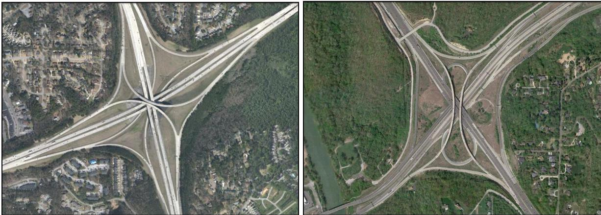
Figure 9 – All Directional Interchange and Directional with Two Loop Ramps
