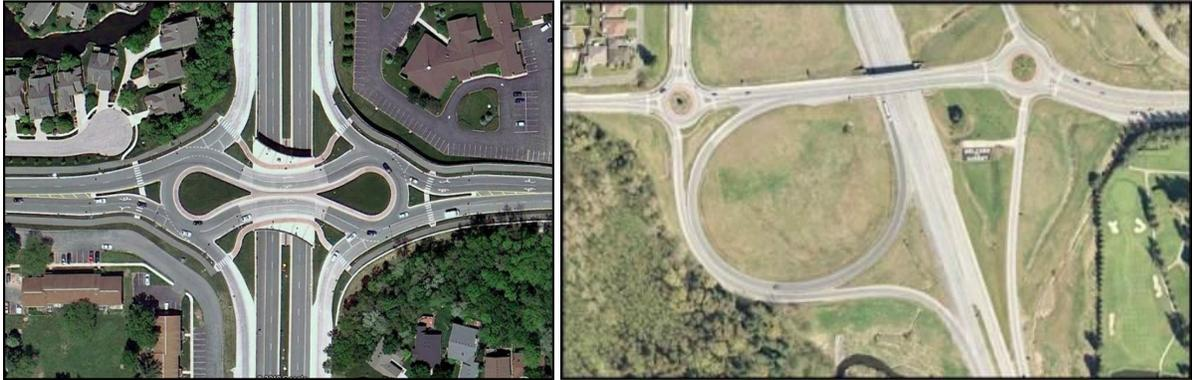
**Figure 14 – Interchanges with Roundabouts**
