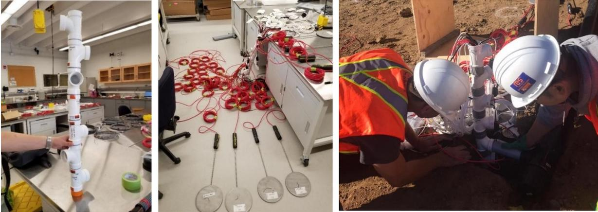
Figure 4 (a) Moisture tree through which all sensors were threaded, (b) Image showcasing how all the sensors were threaded through the moisture tree, (c) installation of the moisture tree on site.
