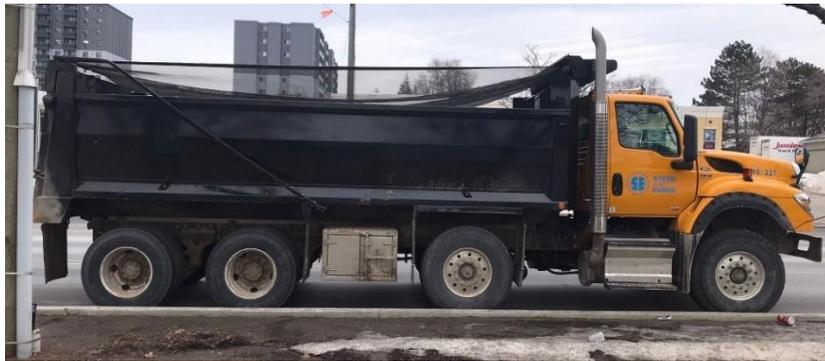
**Figure 6 An image of a truck used for truck testing, with a steering axle, single axle with dual tires and tandem axle with dual tires.**
