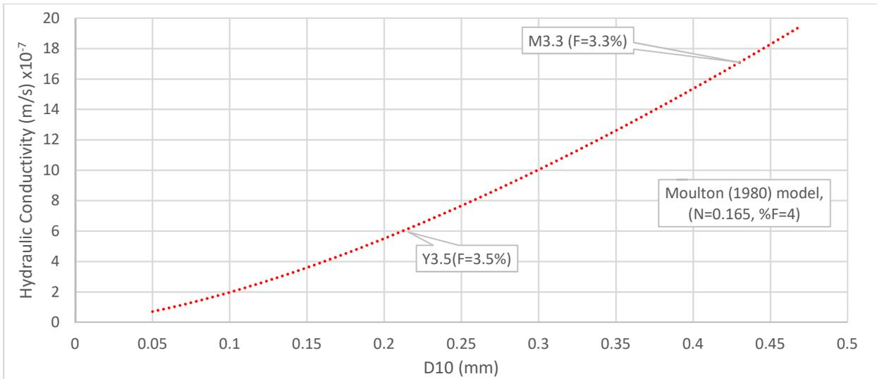
**Figure 7 Sensitivity of Moulton prediction model to the effective size of the blend ( $D_{10}$ )**
