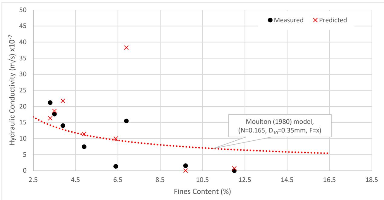
**Figure 6 Effect of fines on the hydraulic conductivity of the tested unbound granular materials**
