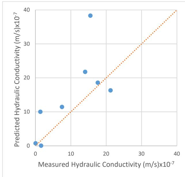
**Figure 5 Measured and predicted hydraulic conductivity using Moulton-1980 equation**
