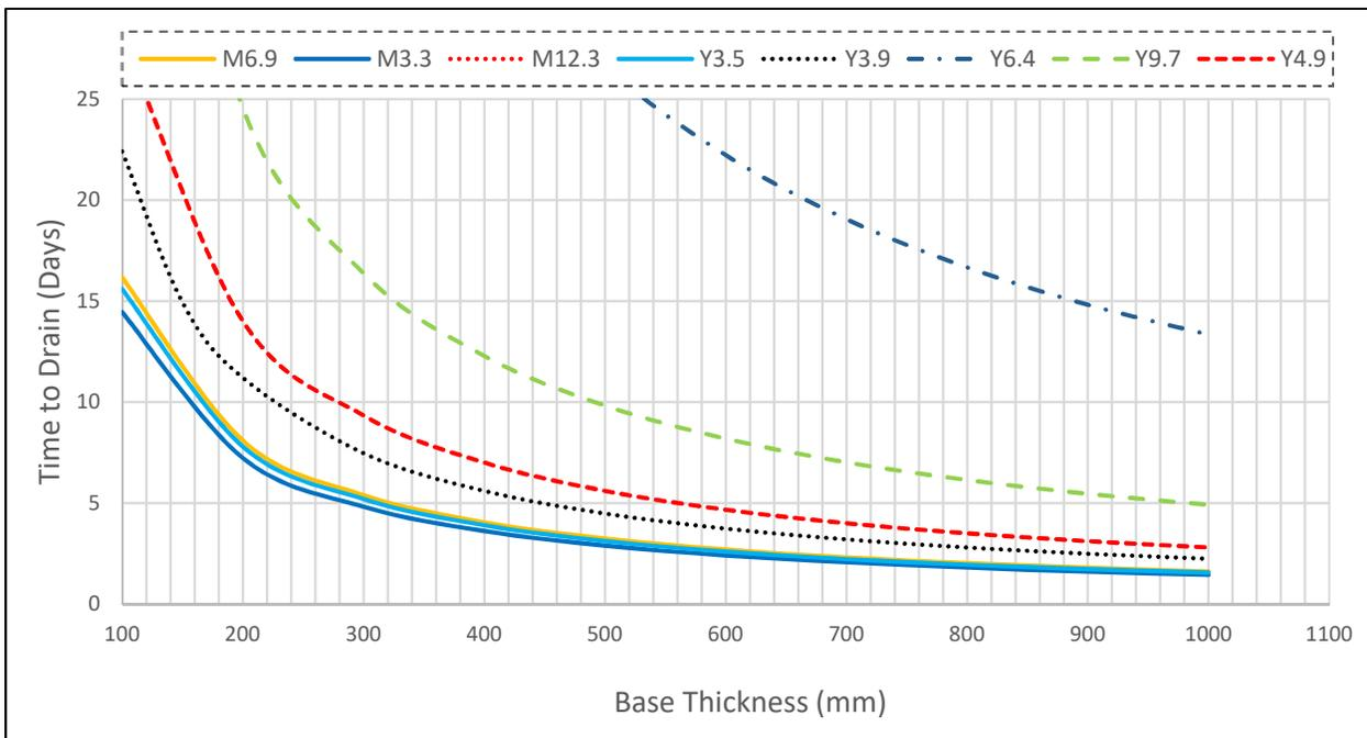
**Figure 8 Relationship between the base thickness and the time required to drain for the tested blends**
