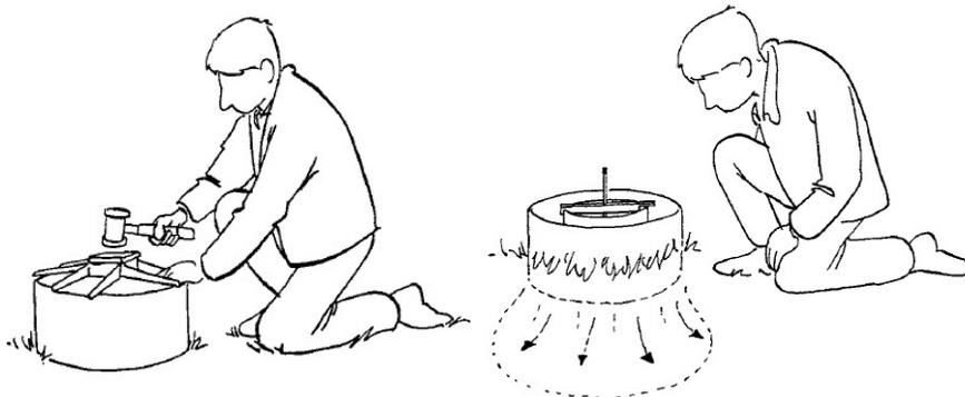
**Figure 4 Setup and operation of the double ring infiltrometer [16]**
