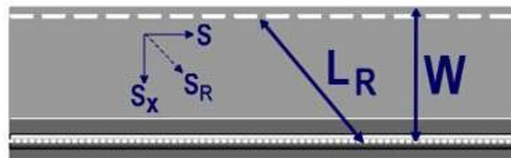
Figure 2 Pavement geometry parameters, (Plan view of a typical pavement surface)
