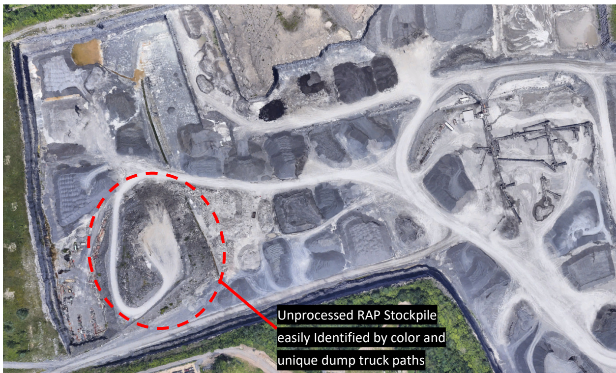
Figure 10 Satellite image of a quarry with RAP stockpile showing that visually identifying crushed RAP stockpile can be more challenging than of unprocessed RAP stockpiles.
