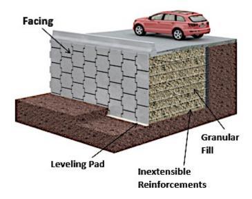
Figure 2 – MSE Wall Components
