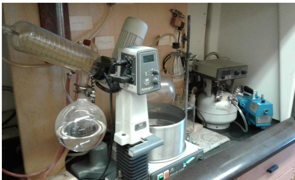
FIGURE 2 Rotary Evaporator Recovery Setup
