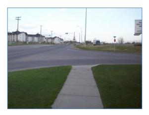
Figure 3: Sidewalk ends abruptly; no continuation on other side of intersection
