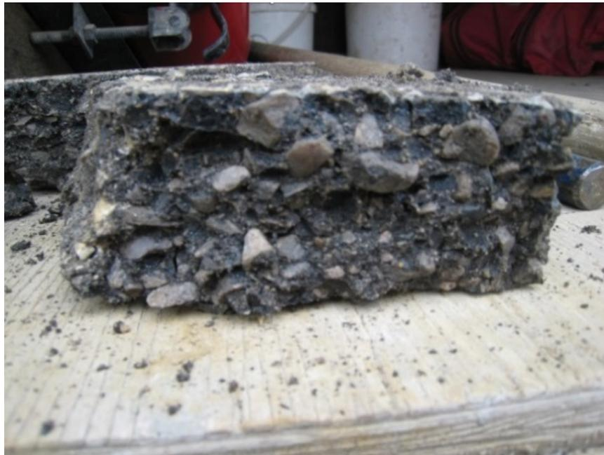
Photograph 1: Asphalt stripping visible in a piece of the asphalt mat obtained from the runway pavement.
