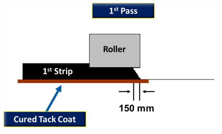
**Figure 10: Unsupported Edge Compaction (Quebec Ministry of Transportation).**
