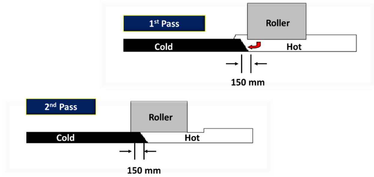
**Figure 11: Supported Edge Compaction (Quebec Ministry of Transportation).**
