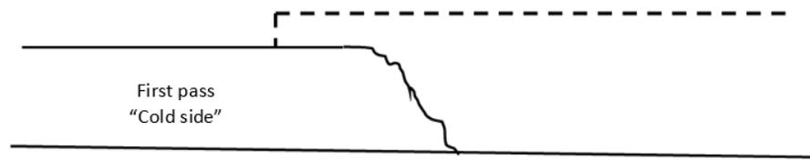
a. Paver laid butt joint
