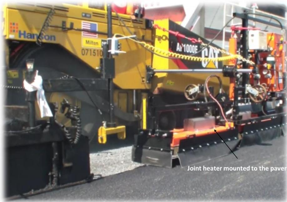
**Figure 8: Joint heater mounted to a paver.**
