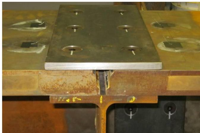
Figure 5: Laboratory prototype of bolted connection of composite steel plate and elastomer decking panels at longitudinal stringer.
