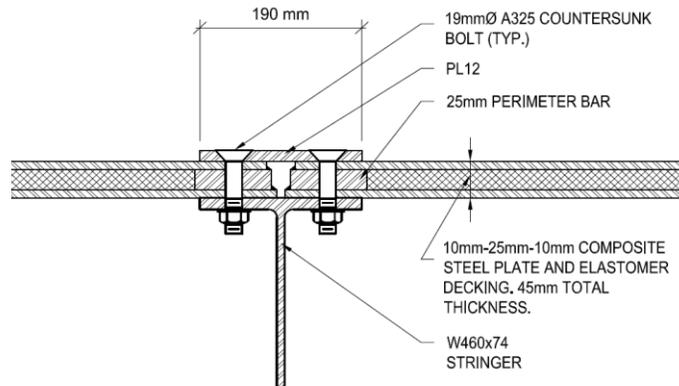
Figure 4: Design drawing of bolted connection of composite steel plate and elastomer decking panels at longitudinal stringer.
