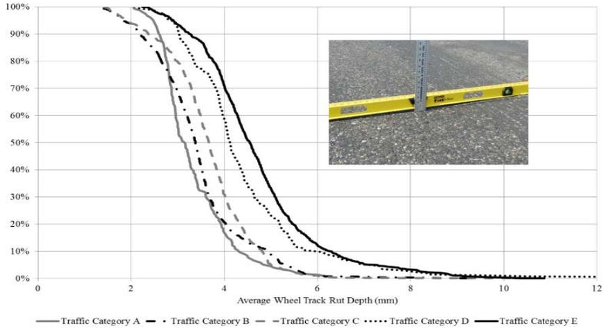
**FIGURE 1 Sensitivity of wheel track rutting to Superpave™ traffic category after seven years of service, based on 147 contracts, 2807 segments (500 lane-m/segment).**
