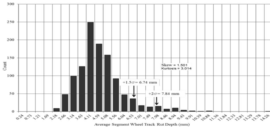
**FIGURE 4 Average wheel track rut depth after 7 years of service based on 64 Superpave™ traffic category D & E contracts, 1125 segments (500 lane-m/segment).**
