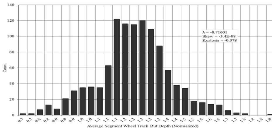
**FIGURE 5 Normalized wheel track rut depth**
