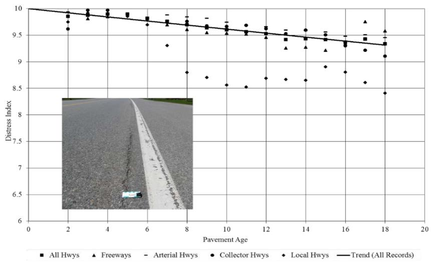
**FIGURE 2 Sensitivity of edge cracking to highway classification, based on 445 contracts.**
