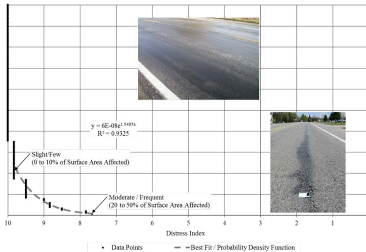
**FIGURE 3 Flushing performance distributions after 7 years of service, based on 445 contracts.**
