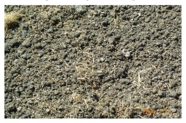
Figure 9 – Geocomposite of Flax Straw and In Situ Material
