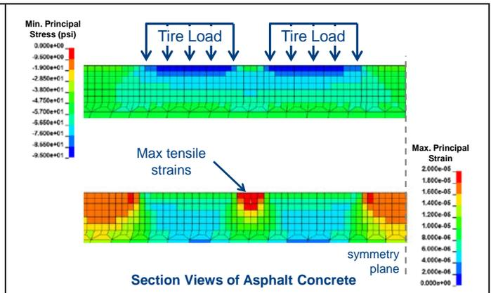
Figure 16. Horizontal Tensile Strains between the Tire Loads
