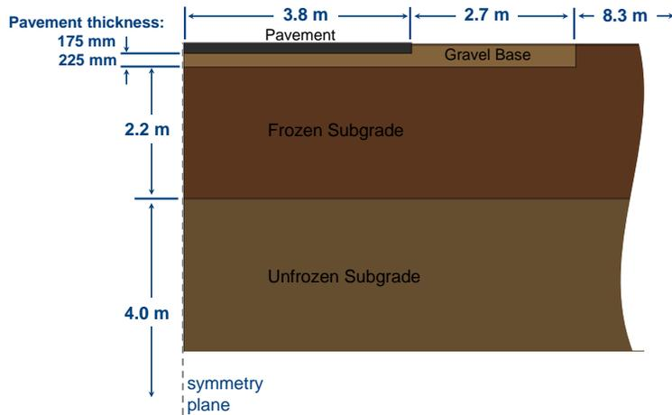
**Figure 14. Road Model Section View for Winter Move**
