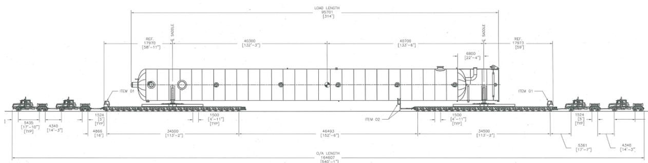
**Figure 13. Proposed Transport Vehicle Configuration for Winter Move**
