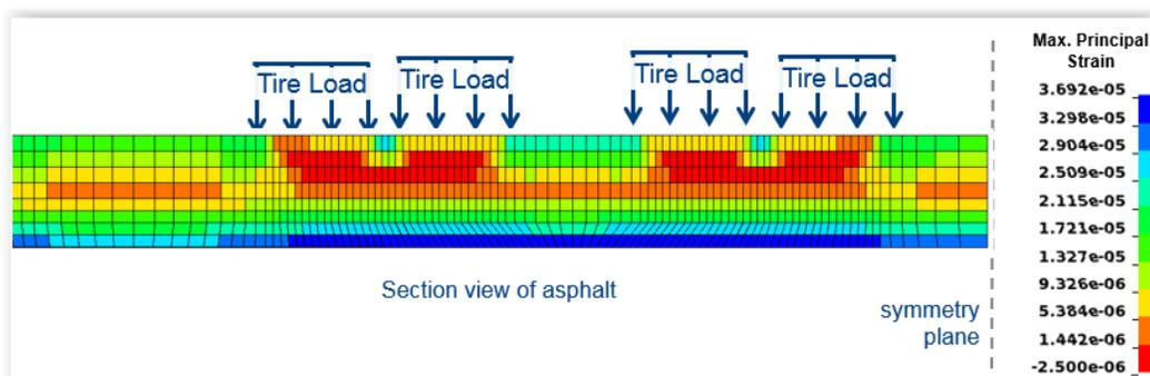
**Figure 11. Horizontal Tensile Strains due to the Upward Pavement Bending**
