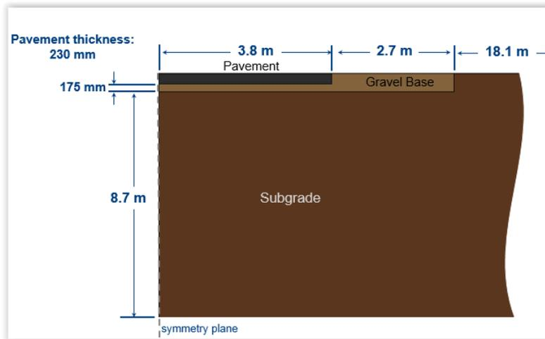
**Figure 4. Road Model Section View for Spring Move**
