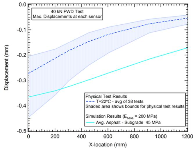
**Figure 5. Falling Weight Deflectometer Simulated Physical Result**
