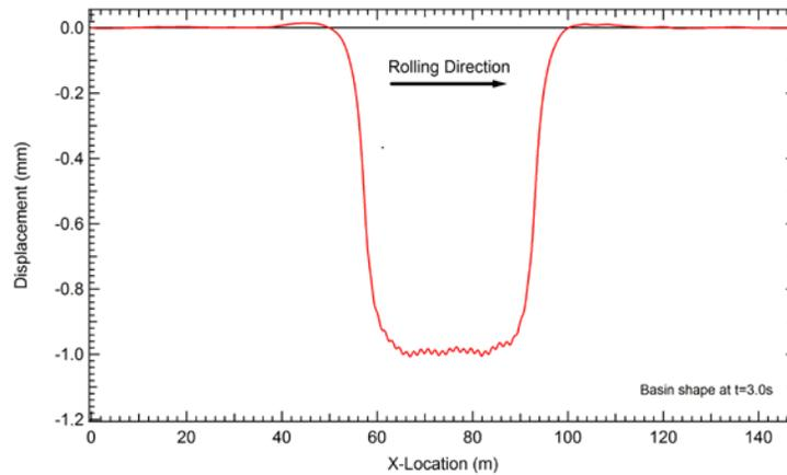
**Figure 8. Roadway Centreline Displacement under Rolling Load**
