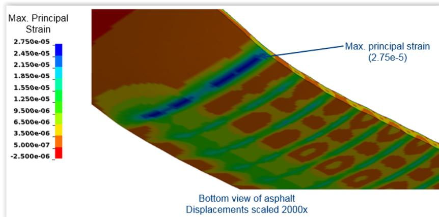
**Figure 10. Horizontal Tensile Strains due to Downward Pavement Bending**
