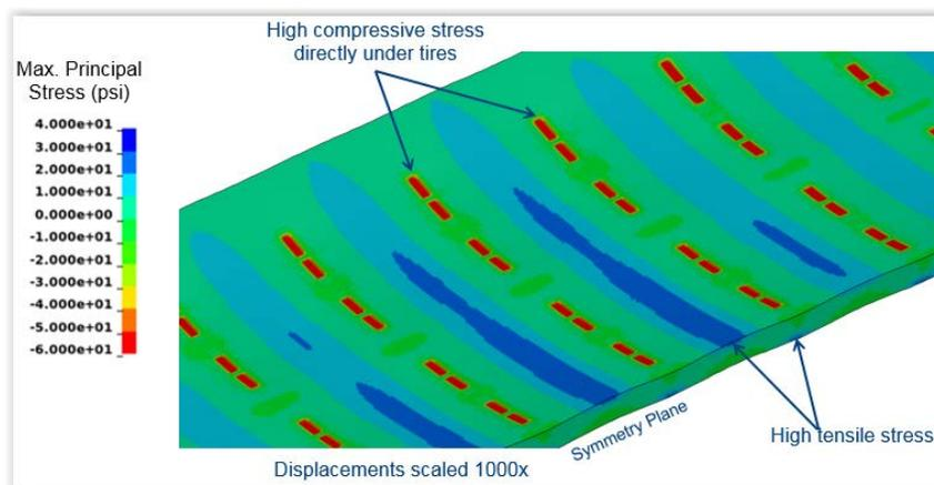
**Figure 9. Stresses at the Bottom of the Asphalt Surface**
