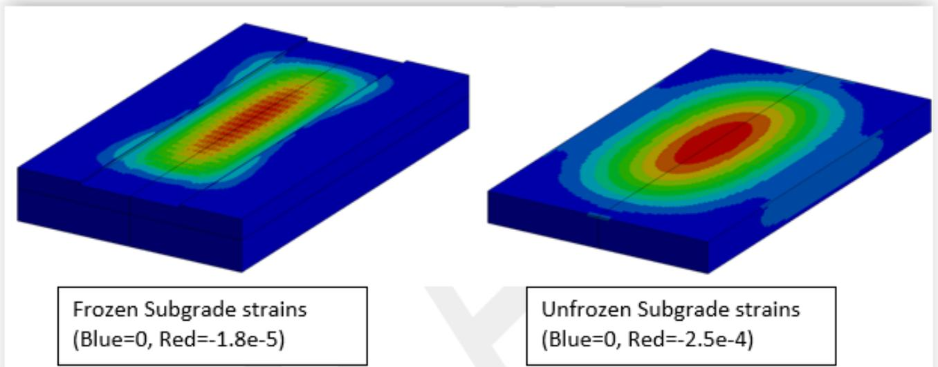
Figure 17. Subgrade Vertical Compressive Strains for Winter Move
