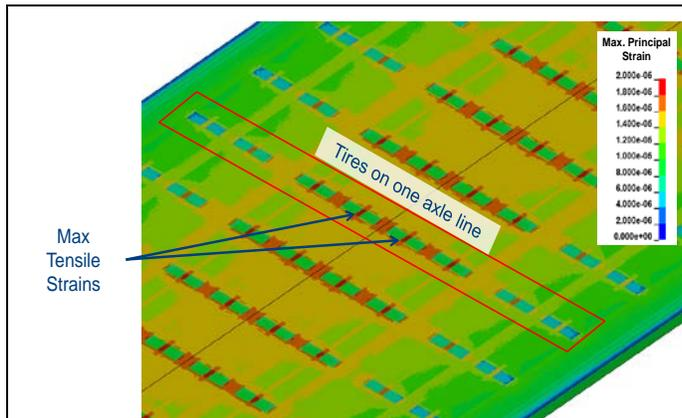
Figure 15. Horizontal Tensile Strains due to the Upward Pavement Bending
