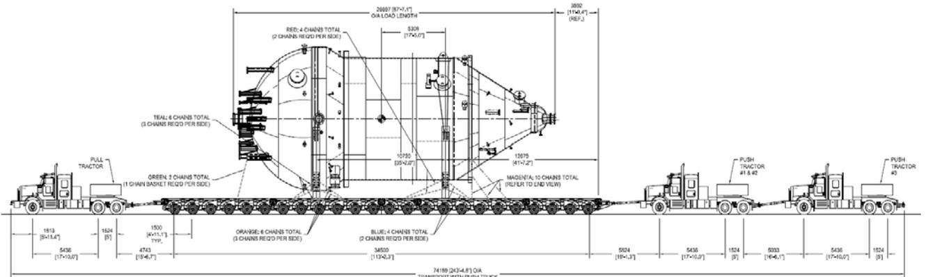
**Figure 3. Proposed Transport Vehicle Configuration for Spring Move**
