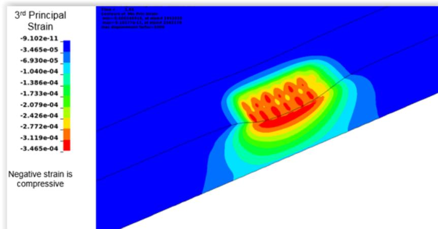
Figure 12. Subgrade Vertical Compressive Strain
