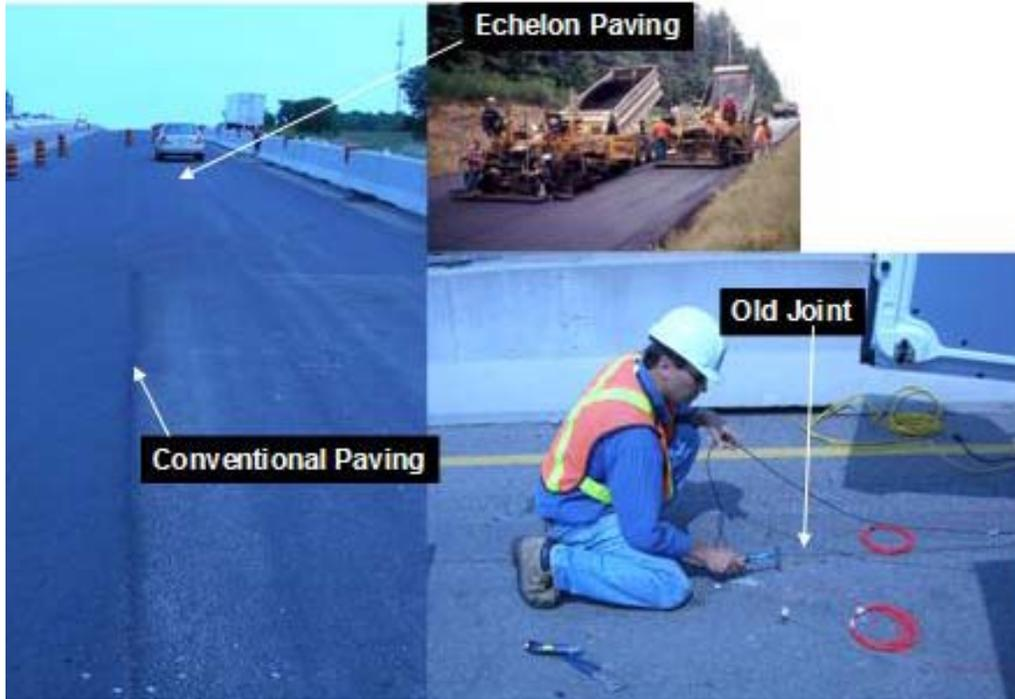
Figure 11 NDT testing of longitudinal joints using seismic waves on Hwy 401
