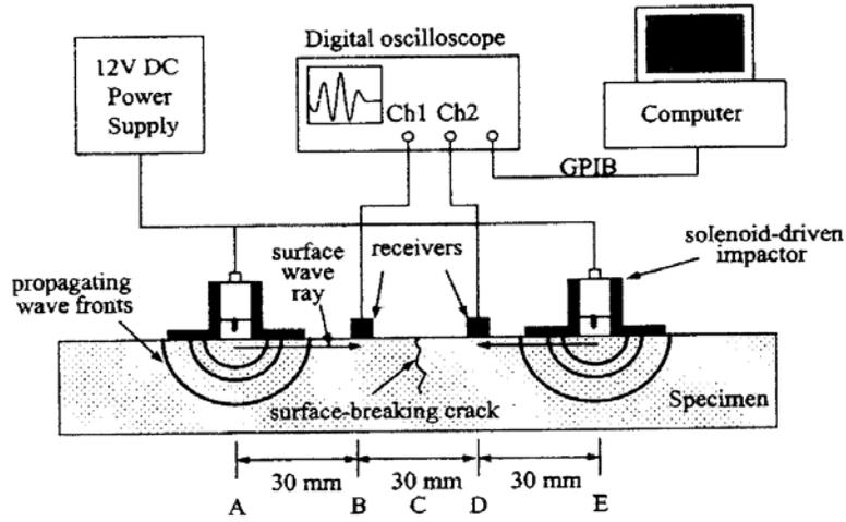
**FIGURE 2** Test set up for the measurement of Transmission Coefficient (TC) (20)
