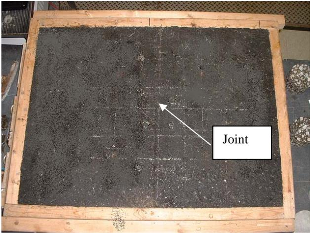
**Figure 5 Laboratory slab specimen with a joint in the middle within the molding frame**
