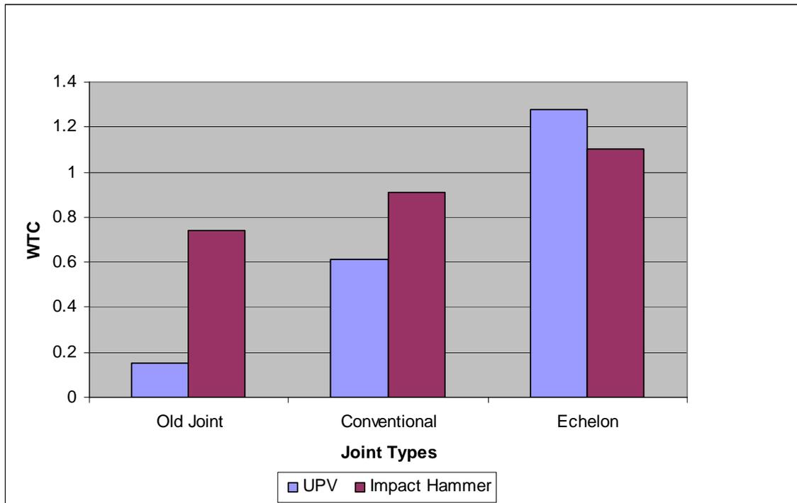
Figure 12 Seismic wave based NDT test results - Hwy 401
