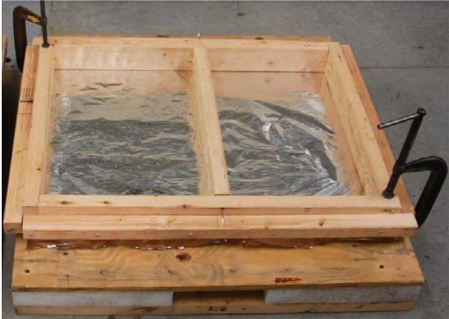
**Figure 4 Molding frame used for laboratory slab specimen before placing the mix**
