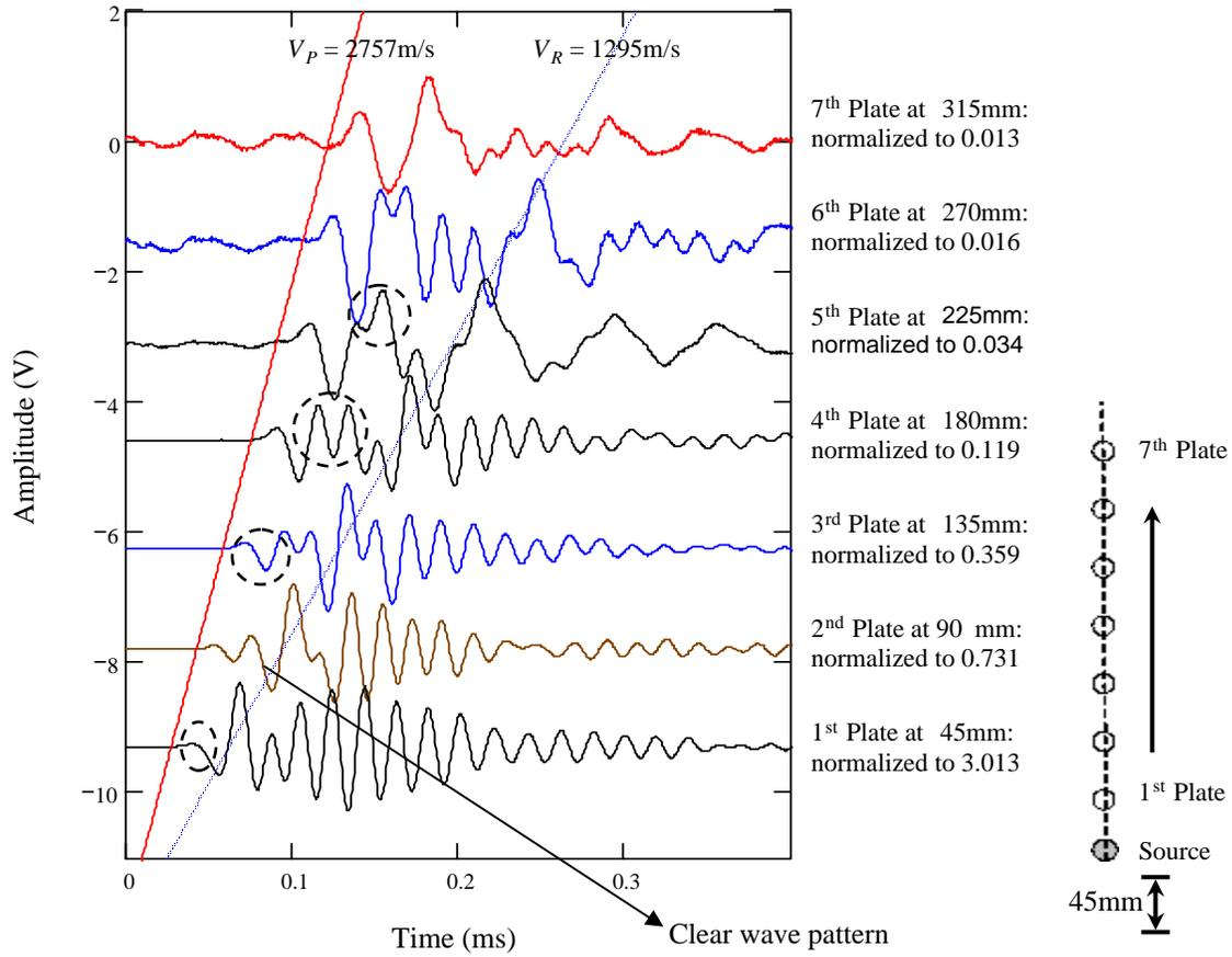
**FIGURE 9** Ultrasonic wave signals received at the seven locations along the linear testing geometry - the dotted circles mark the wave interference
