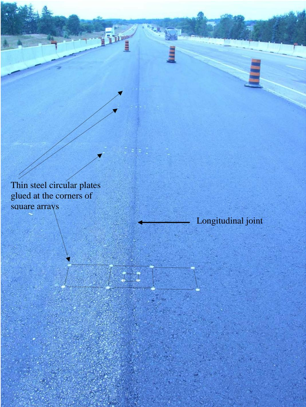
**Figure 10 Thin steel plates were glued across the joint prior to testing on Hwy 401**
