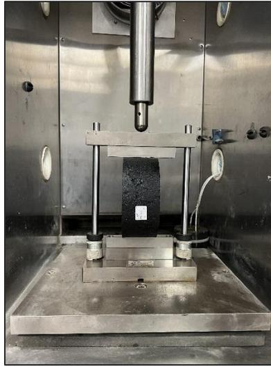
**Figure 5: IDEAL-CT test setup**
