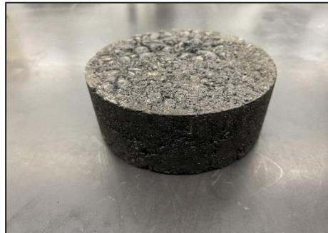
**Figure 4: A Superpave gyratory compacted test specimen for IDEAL-CT**
