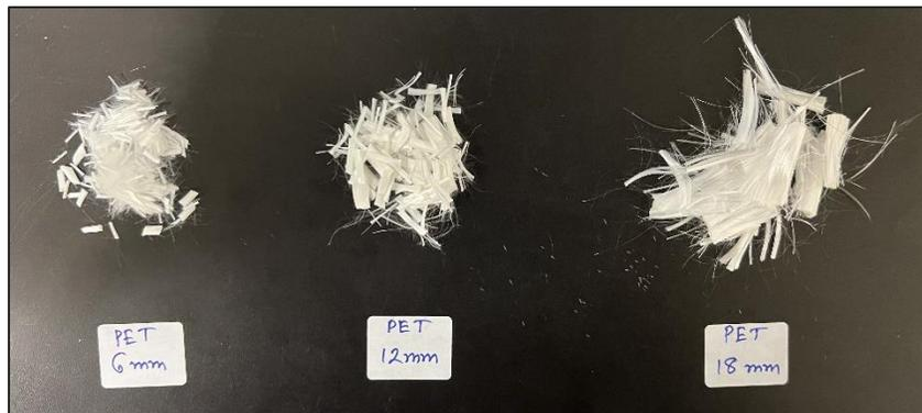
**Figure 3: PET fibres in different lengths (6 mm, 12mm, 18 mm)**
