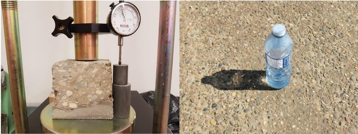
Figure 8 (left): Block cut from Curries Landing Road in 2018. Figure 9) Wearing surface of CLR during the 5<sup>th</sup> year of road life, summer of 2019. The road maintains a well-bound pebbled surface. Wearing surface is 20cm thick and comprised of A-base aggregate plus Penner clay mixed to ~32% -200 mesh fines resulting in ~10% clay minerals in the final mix.
