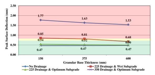
Figure 7 Collector Roadway Comparisons (80mm AC, Type CH Subgrade)
