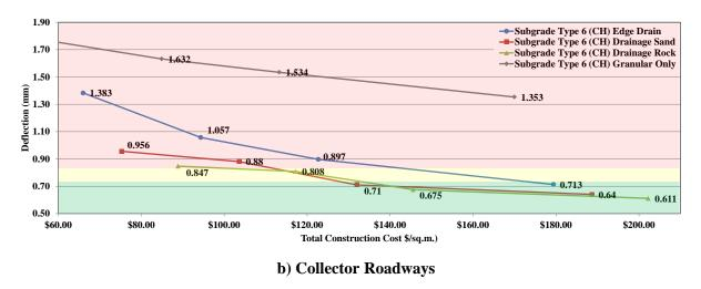
Figure 5 Total Construction Cost vs. Peak Surface Deflection – Subgrade Type CH
