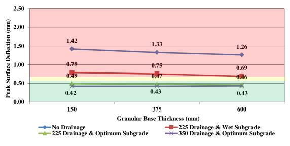
Figure 8 Arterial Roadway Comparisons (110mm AC, Type CH Subgrade)
