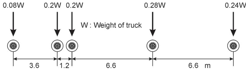
Figure 1 – CSA-S6-14 CL-W truck axle configuration
