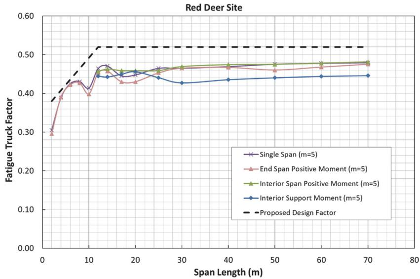
Figure 7 – Adjusted fatigue truck factors for Red Deer Site (CL-800 truck)
