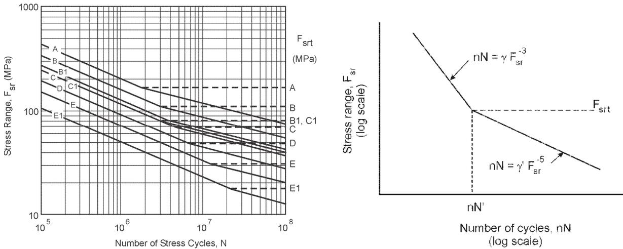
Figure 2 – CSA-S6-14 Fatigue Curves
