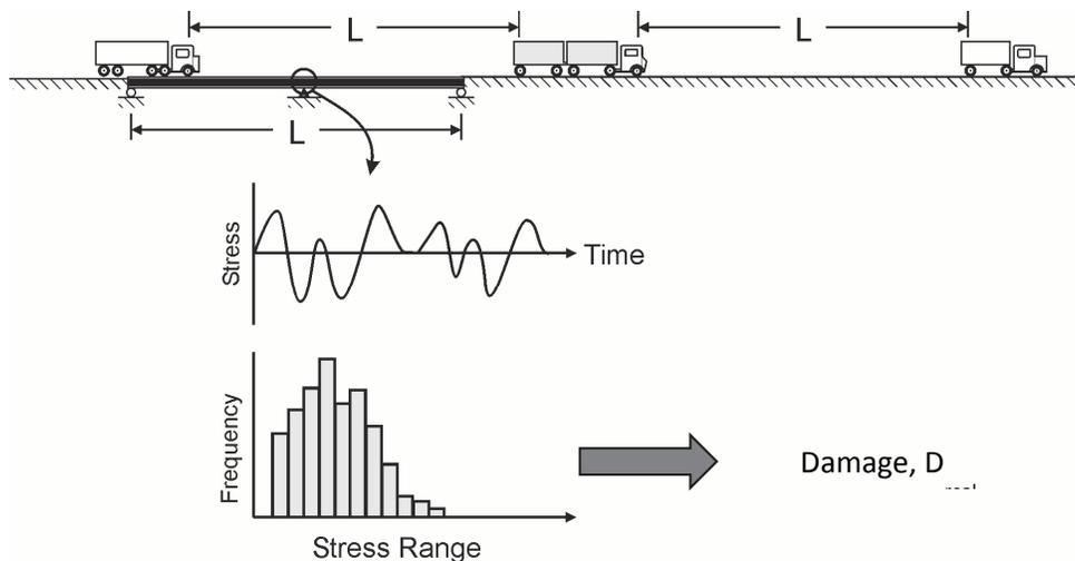
Figure 3 – Schematic of the calibration process
