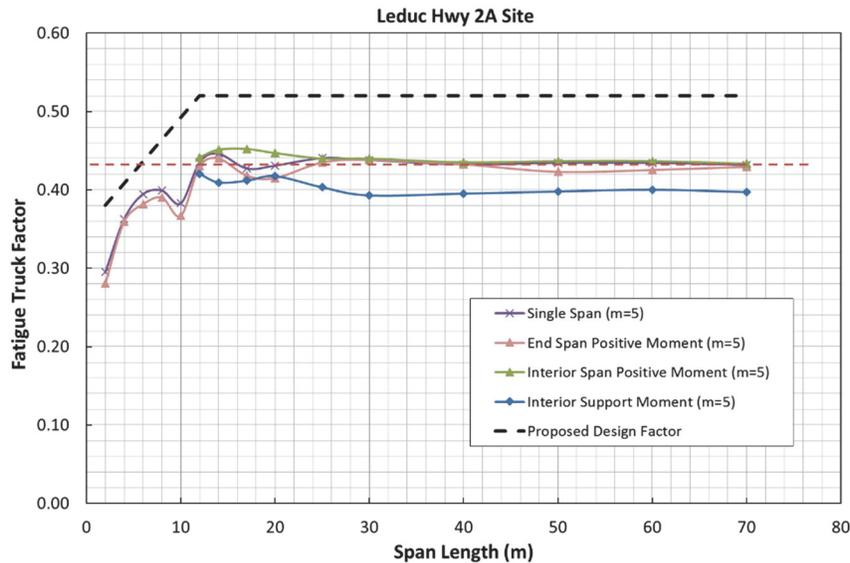
Figure 9 – Adjusted fatigue truck factors for Leduc Hwy 2A Site (CL-800 truck)
