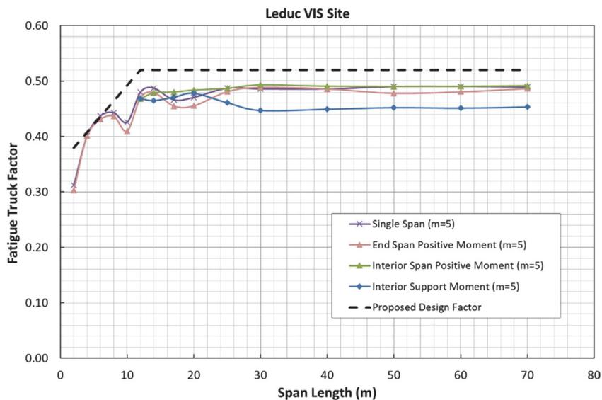
Figure 8 – Adjusted fatigue truck factors for Leduc Hwy 2 Site (CL-800 truck)
