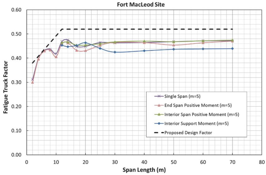
Figure 10 – Adjusted fatigue truck factors for Fort MacLeod Site
