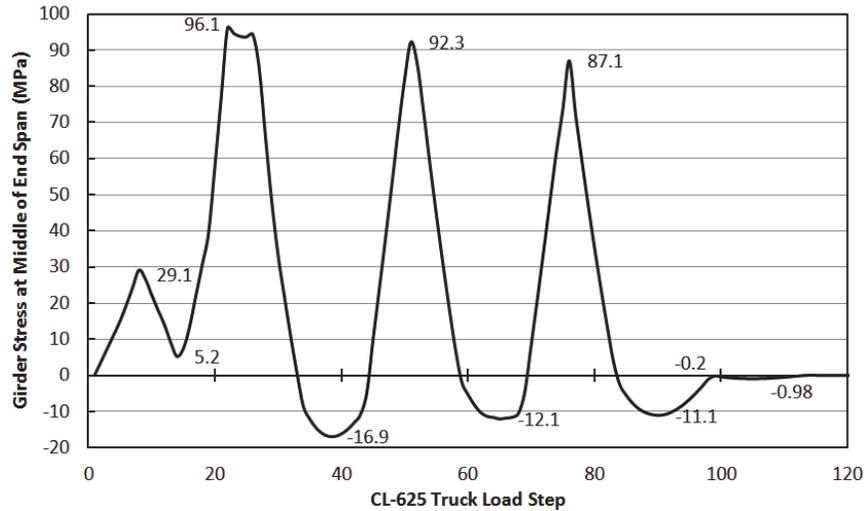
Figure 5 – Typical Stress History in Exterior Span of Four-Span Girder (Span Length = 4 m)
