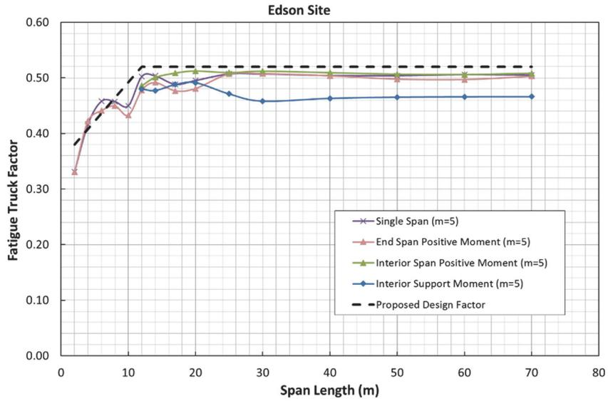
Figure 11 – Adjusted fatigue truck factors for Edson Site
