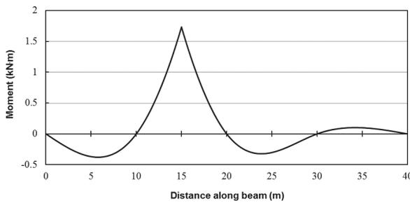
(c) Interior Span Positive Moment – 4-span continuous
