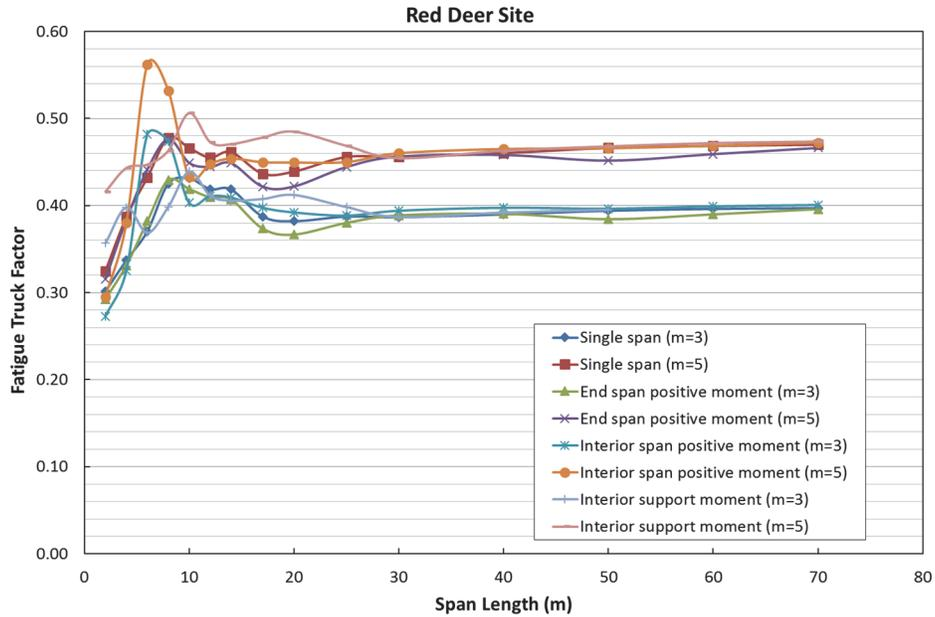
Figure 6 – Calibration factors for Red Deer Site (CL-800 truck)
