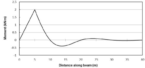
(b) End Span Positive Moment – 4-span continuous
