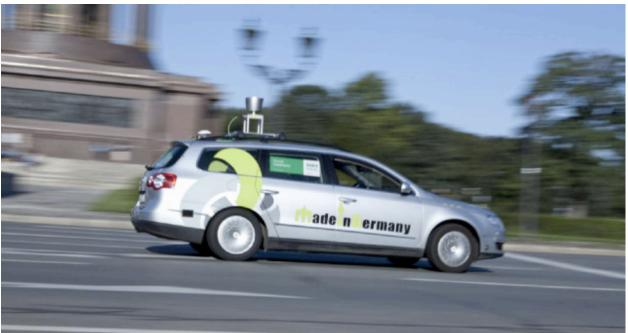
Figure 3 The AutoNOMOS Labs 'MadeInGermany' autonome
