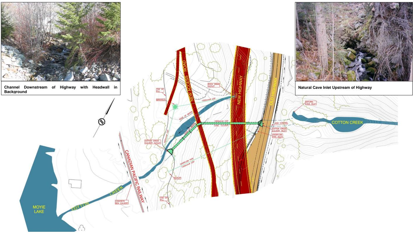
FIGURE 3 – PLAN VIEW OF COTTON CREEK CULVERT DESIGN
