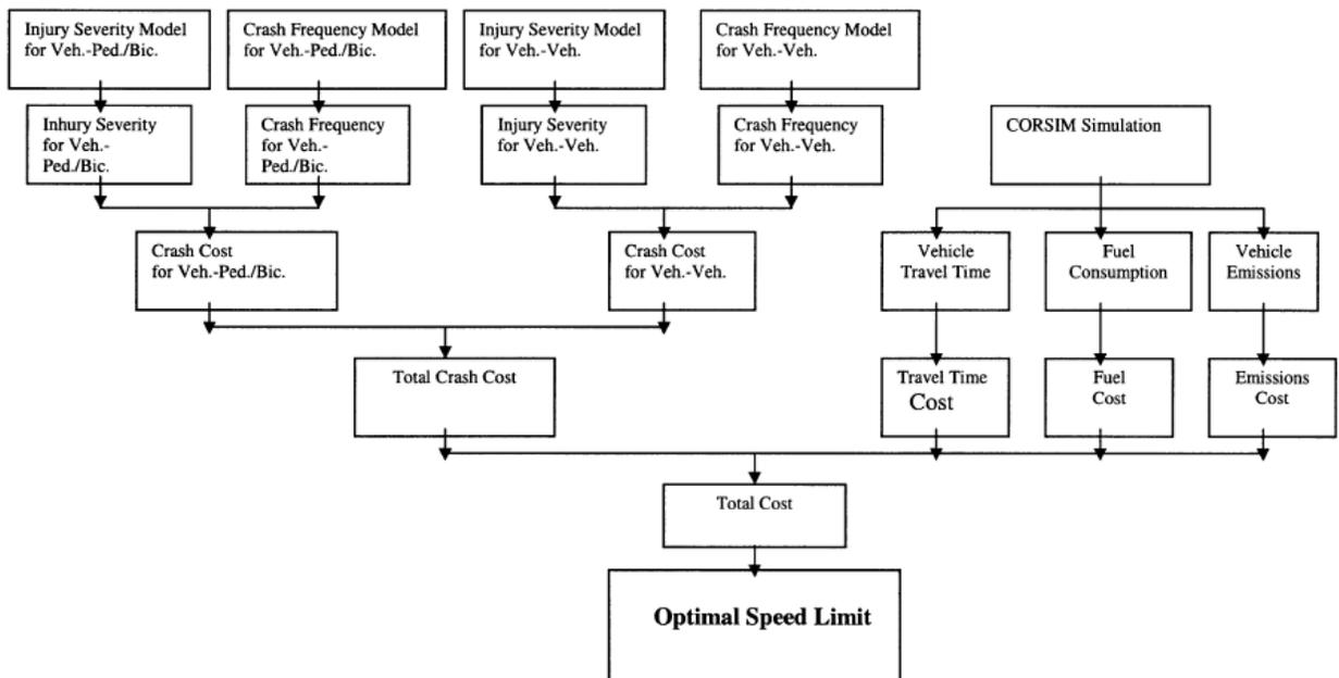
FIGURE 4: Process for Setting Optimal Speed Limits (Source 12)
